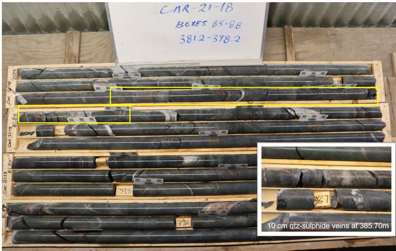
Figure 6. Drill core intercept showing several quartz-carbonate sulphide veins cutting through mafic volcanics. Significant gold intercept at 6.88 gpt Au/ 1.50m (from 384.5m) including 19.60 gpt Au / 0.50m.
