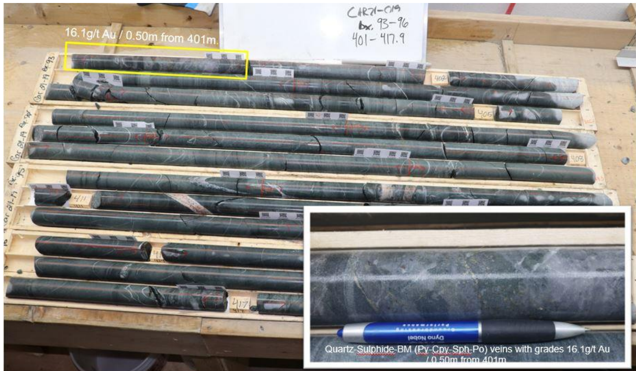
Figure 7. Drill core intercept showing quartz-carbonate sulphide veins in mafic volcanics. Significant gold intercept at 5.84 gpt Au / 1.50m (from 400.0m) including 16.10 gpt Au / 0.50m.
