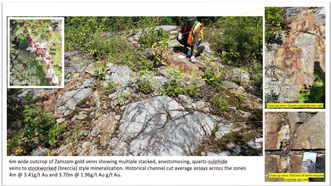
Figure 10: Outcrop section showing a 6m zone with multiple stacked quartz-sulphide veins enveloped by stockworked (breccia) mineralization at Zamzam gold zone.
