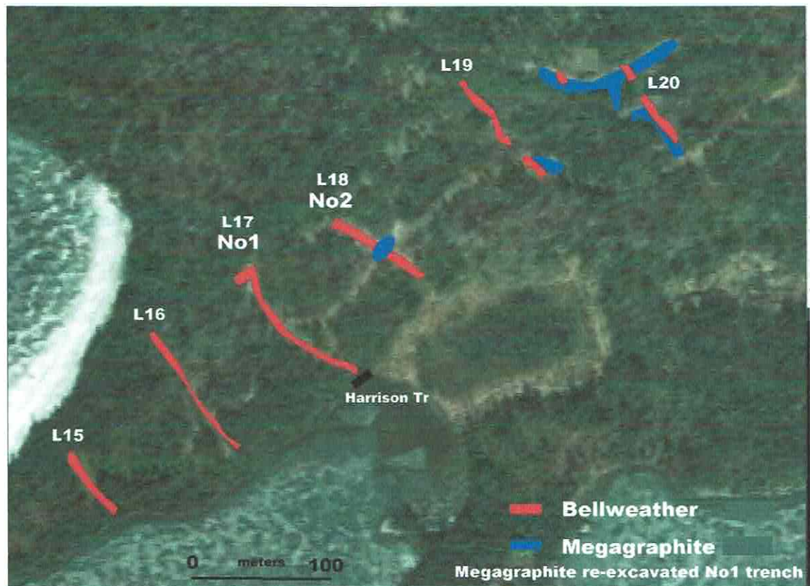
Figure 16. Location of trenches excavated by Mega Graphite in 2012 related to Bellwether 1988 trenches in the Harrison Graphite Showing area.
