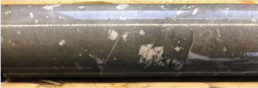
Photo 2: Core sample of the Feldspar-Phyric Basalt. NQ drill core 4.6cm diameter. From DDH D1-19-4 at 90m.
