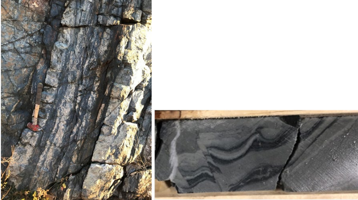
Photo 5: Typical well bedded sequence of mudstones and siltstones. Left: from a Trans-Canada Highway Roadcut north of Eureka. Right: NQ drill core sample from drill hole D1-19-05 near the colar.
