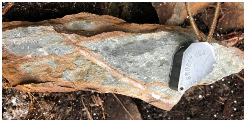
Photo 14: Quartz-ankerite-pyrite veinlet in mafic volcanics from the Wedge Gold Occurrence. Note the rusty brown weathering of the ankerite on the weathered surface and at the veinlet contacts. Outcrop D1-AT-20-60 (0.4 g/t Au). Coordinates 284885E 5385808N
