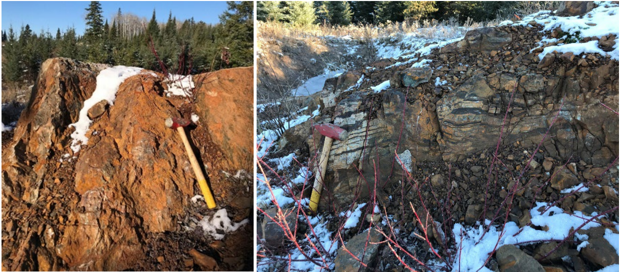
Photo 12: Kasper Gold occurrence. To the left, a sulphidic chert looking west (grab sample 8.72 g/t Au). To the right, the spatially associated banded iron formation at Kasper looking north (grab sample 0.08 g/t Au).
