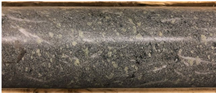
Photo 6: Core sample of typical unaltered feldspar-amphibole phyric intermediate intrusive.
