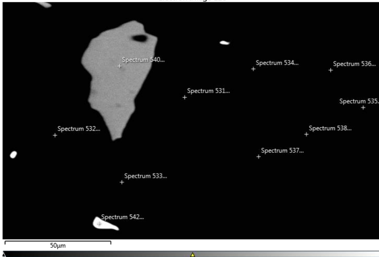
Brightness reduced further to show Ni-Co-Fe-S (spectrum 540) and Ni-Fe-Sb-S-S (spectrum 542).
