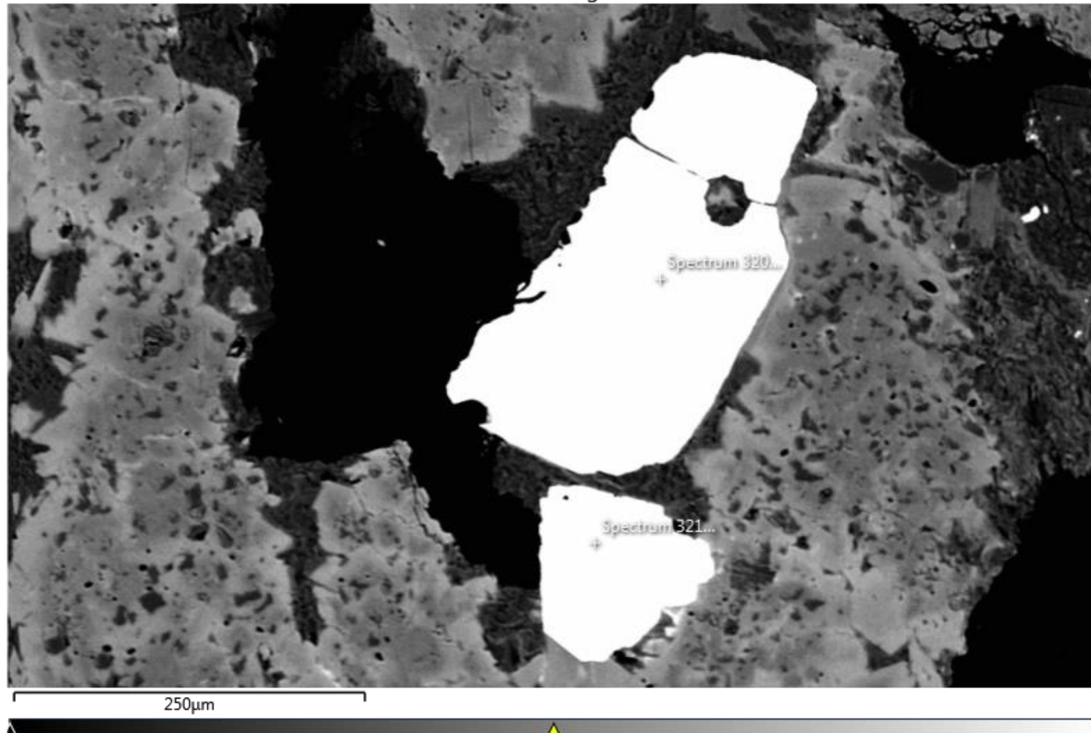
Backscatter image illustrating a groundmass of compositionally variable dolomite-ankerite solid solution carbonate hosting grains of chromite (spectrum 320) and Ni-As-Sb-Co-S (spectrum 321).
