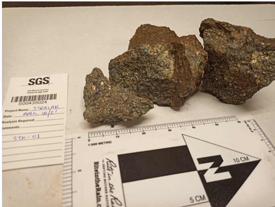
Photo 6 – Sample S00435024 from East Zone 10.55% Zn, 0.36% Cu, 0.17% Pb, 0.57oz/t Ag, 0.02 g/t Au
