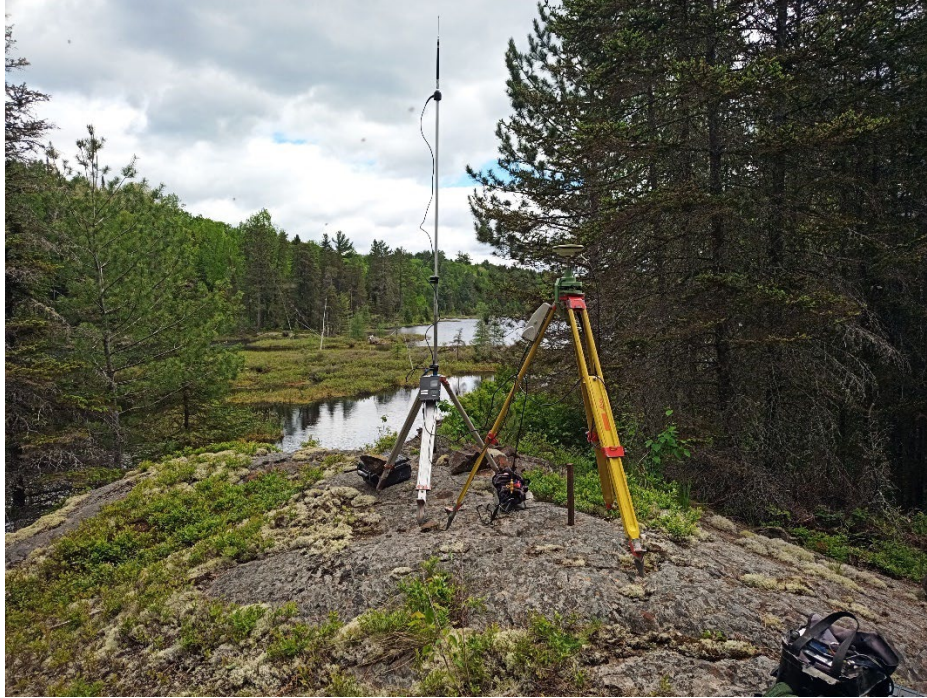
Photo 5 – GPS Base Station setup over Control Point No.1
