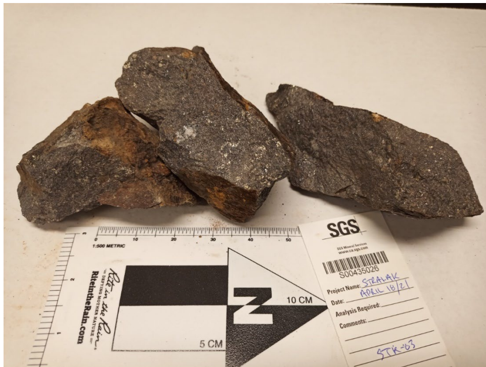
Photo 7 – Sample S00435026 from West Zone 16.53% Zn, 0.03% Cu, 4.29% Pb, 10.48 oz/t Ag, 0.13 g/t Au
