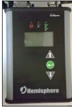
Figure 14: Hemisphere R330 GPS receiver.
