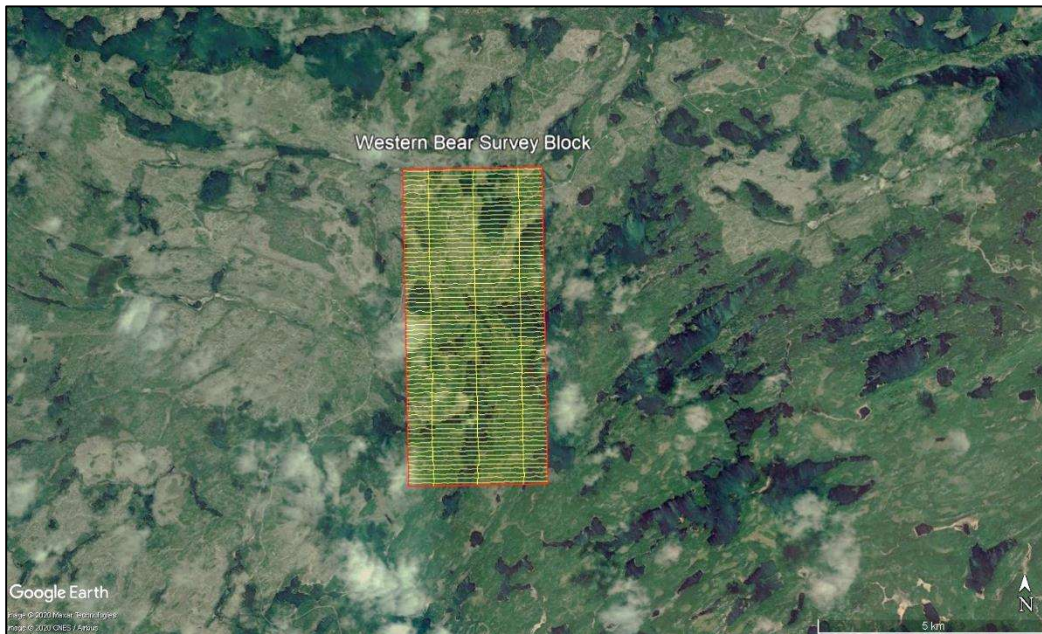
Figure 3: Plan View – Western Bear survey block with actual flight lines in yellow and survey block boundary in red.
