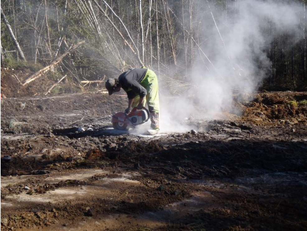
Figure 10: Geotech cutting a channel sample
