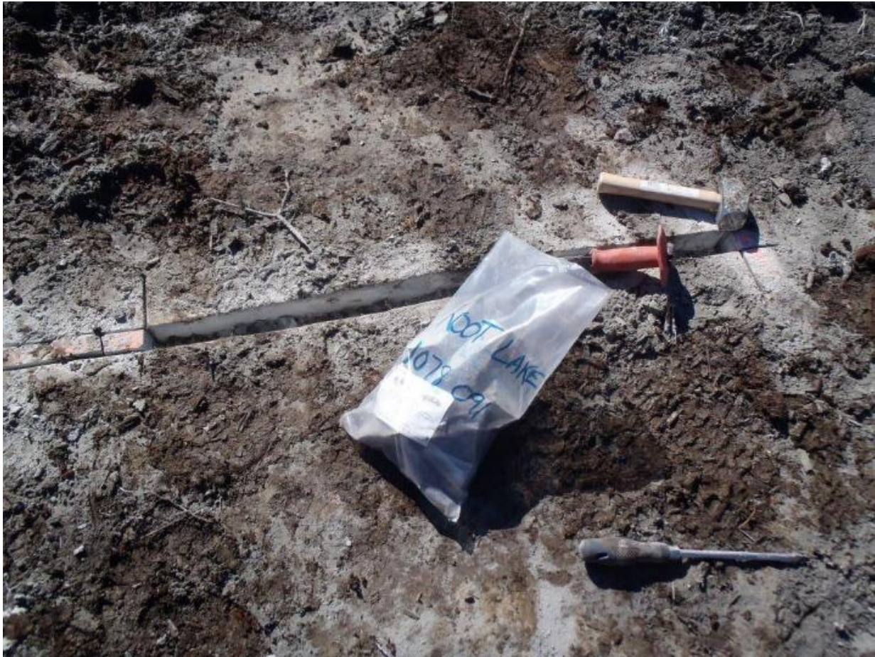
Figure 13: Strip #2 Channel Sample Cut and Bagged with its tag#
