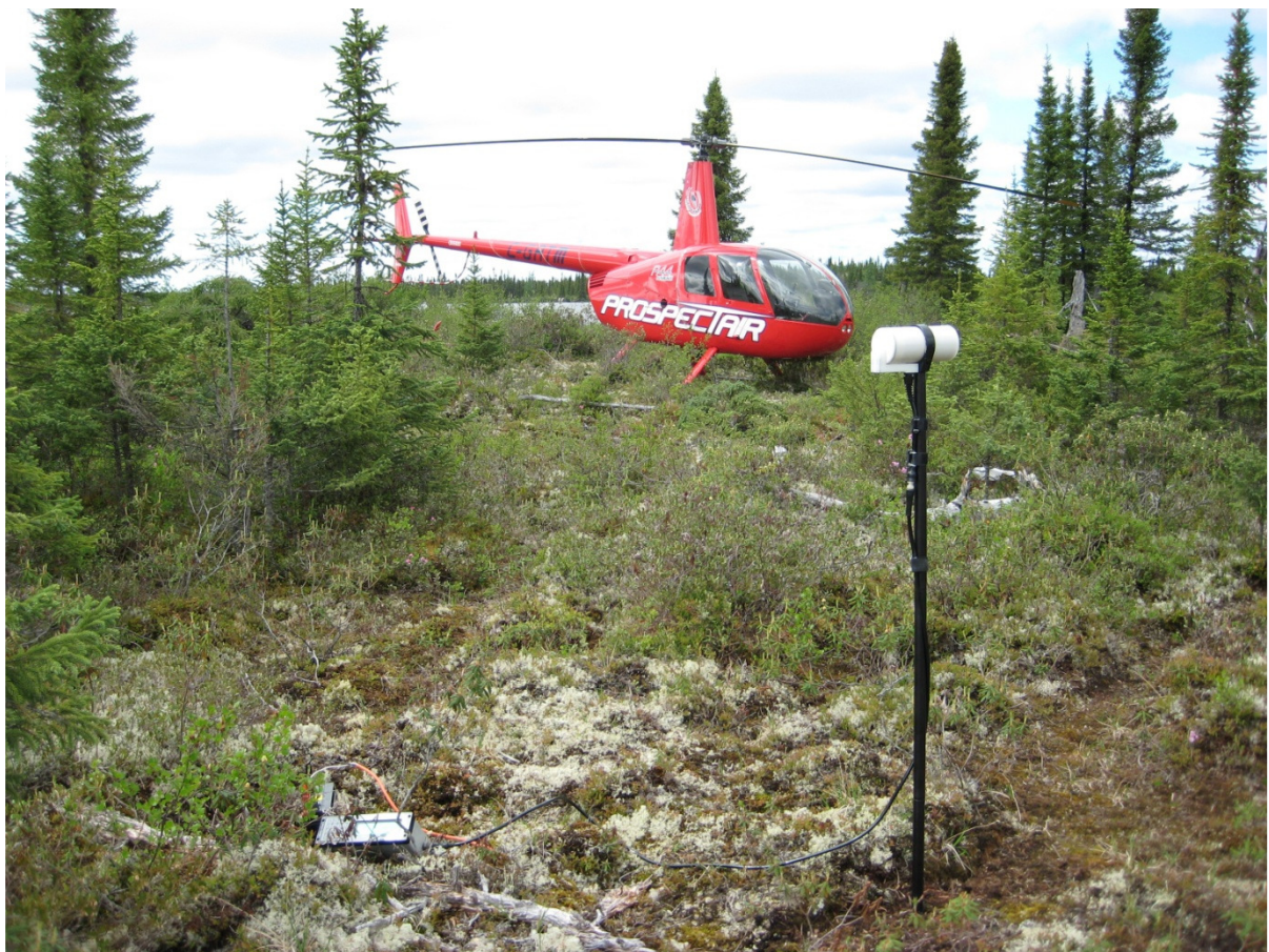
Figure 5: Example of a magnetic base station setup
