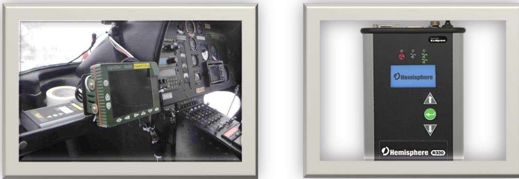
Figure 9 – AgNav main console (left) and Tee-Jet GPS receiver (right).
