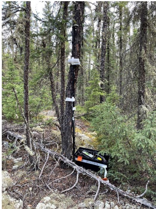
Figure 8 – Base station magnetometer used for diurnal corrections.
