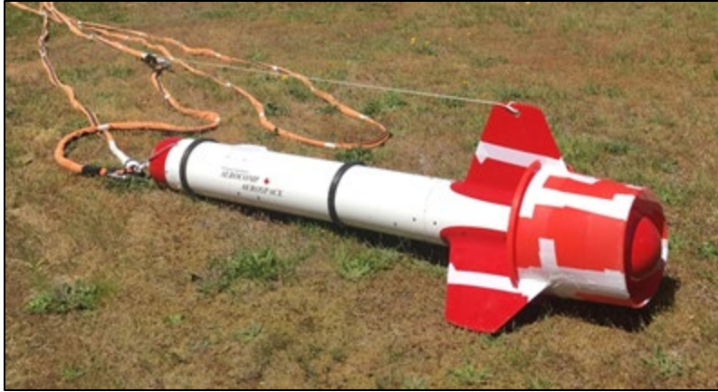
Figure 7 – Airborne magnetometer housing with tow cable.
