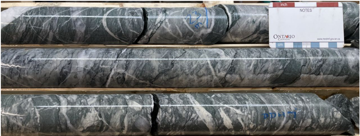
Photo 18: Typical Green Breccia from drill hole D1-21-7 at 23 to 26m.
