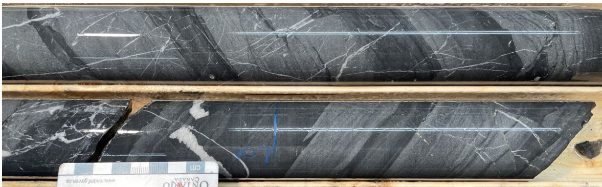
Photo 5: Typical well bedded sequence of mudstones and siltstones from drill hole D1-21-14 at 107m. Minor sandstones are also present.
