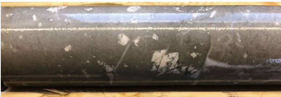
Photo 1: Core sample of the Feldspar-Phyric Basalt. NQ drill core 4.6cm diameter. From DDH D1-19-4 at 90m.
