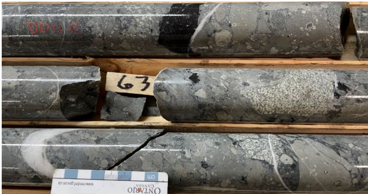
Photo 8: Polymictic conglomerate from drill hole D1-21-12 at 63m. The conglomerate could be considered a polymictic breccia as fragments are rounded to angular and very poorly sorted. A great variety of fragments types are observed including feldspar-phyric basalts, black shale, sandstone and diorite.
