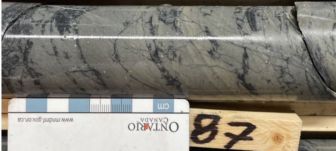
Photo 4: Intensely altered sandstone showing remnants of bedding in drill hole D1-21-13 at 87m. The sample is located within an interval of 0.83 g/t Au over 6m.
