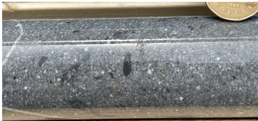
Photo 7: Coarse grained polymictic sandstone (wacke) from drill hole D1-21-14 at 188m.
