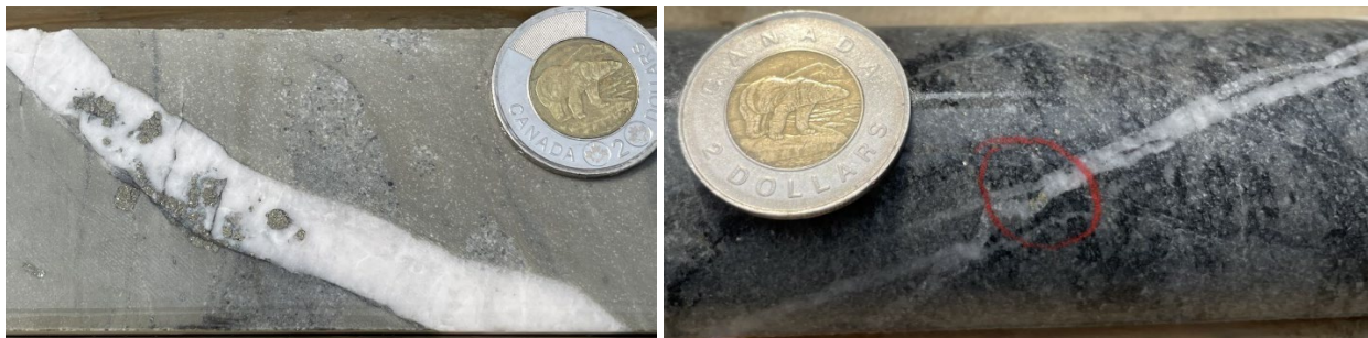
Photo 27: Gold Mineralization. Left: Quartz-ankerite-pyrite veinlet in sandstone from drill hole D1-21-10 at 79.9m. This single veinlet is responsible for an assay of 0.78 g/t Au over a 1 metre interval from 79m to 80m. Right: Quartz-ankerite-pyrite veinlet in sandstone from drill hole D1-21-10 at 102.3m with a speck of visible gold. This single veinlet is responsible for an assay of 2.9 g/t Au over a 1 metre interval from 79m to 80m.
