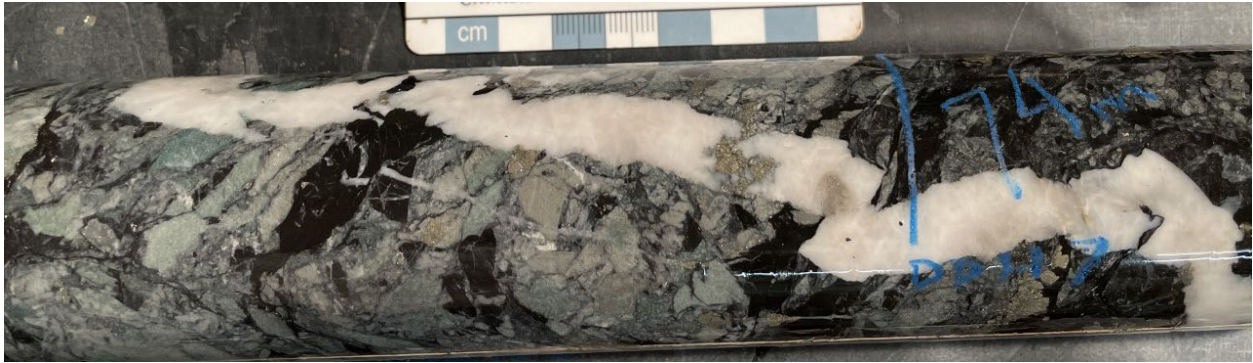
Photo 29: Quartz-ankerite-pyrite veinlet in heterolithic, black-matrix breccia from drill hole D1-21-7 at 74m. This single veinlet is responsible for an assay of 0.6 g/t Au over a 1 metre interval.
