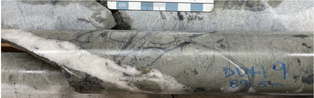
Photo 28: Quartz-ankerite-pyrite veinlet in highly altered sandstone from drill hole D1-21-9 at 89.5m. This veinlet along with three others is responsible for an assay of 3.8 g/t Au over a 1 metre.
