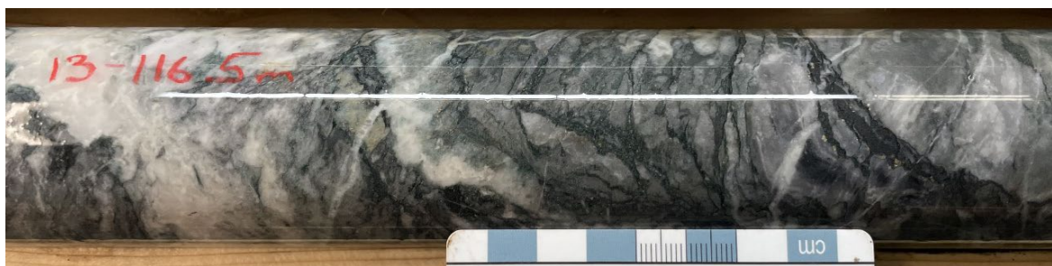
Photo 20: Typical Green Breccia from drill hole D1-21-13 at 116.5m. Here the Green Breccia locally shows jigsaw-puzzle textures and shows several generations of quartz-calcite and quartz-chlorite veinlets.
