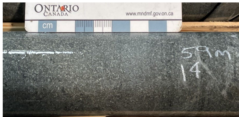
Photo 11: Core sample of fresh diorite from drill hole D1-21-14 at 59m.
