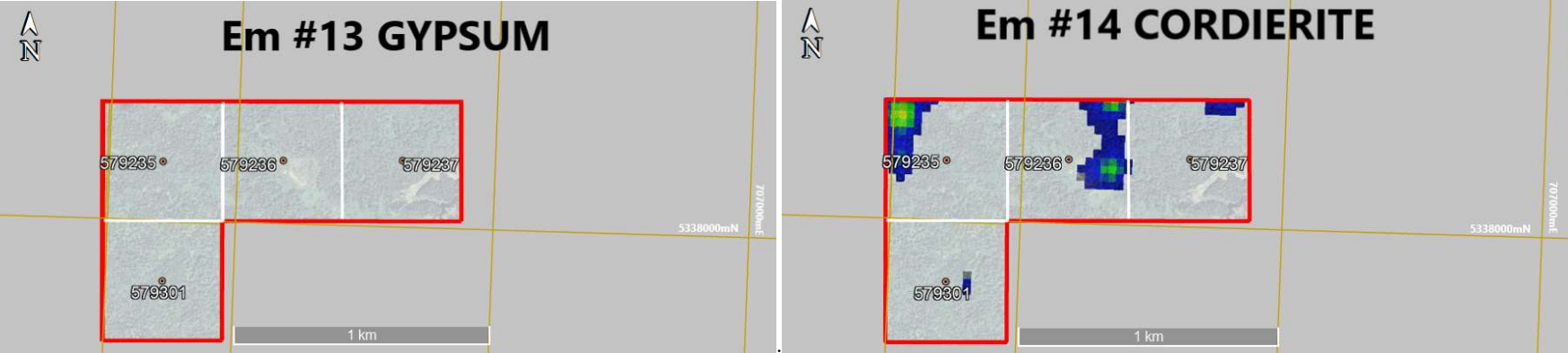
Figure 7.7 Long Wave Infrared Survey: Gypsum & Cordierite Abundance Maps
