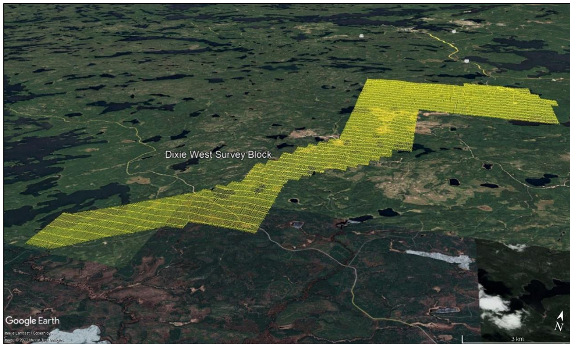
Figure 4: Terrain View – Dixie West survey block with actual flight lines displayed in yellow.
