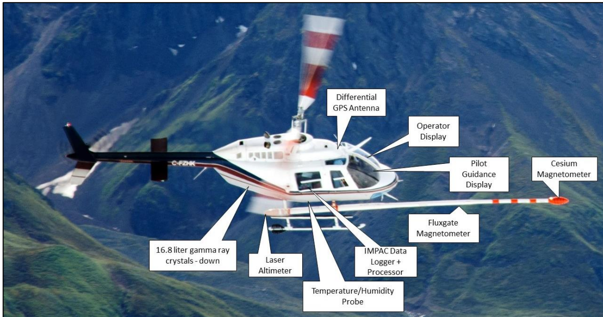
Figure 6: Survey helicopter equipped with a magnetic sensor and gamma spectrometer. Magnetic data were not collected for this survey.
