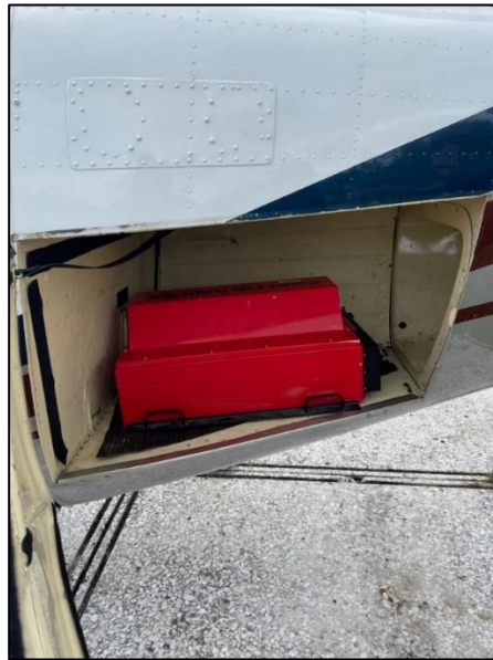
Figure 12: Medusa gamma spectrometer system with four downward detectors; 16.8 litres in total.
