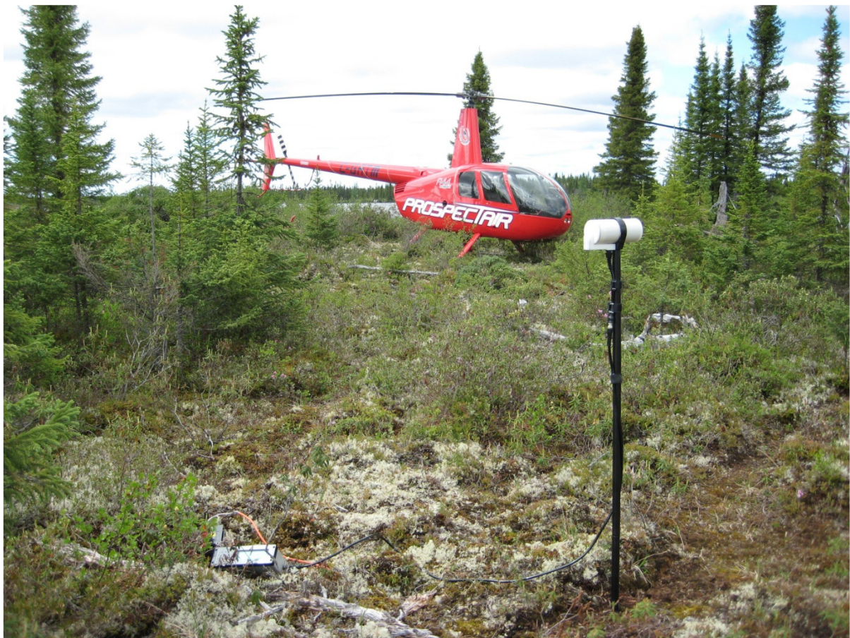
Figure 6: Example of a magnetic base station setup
