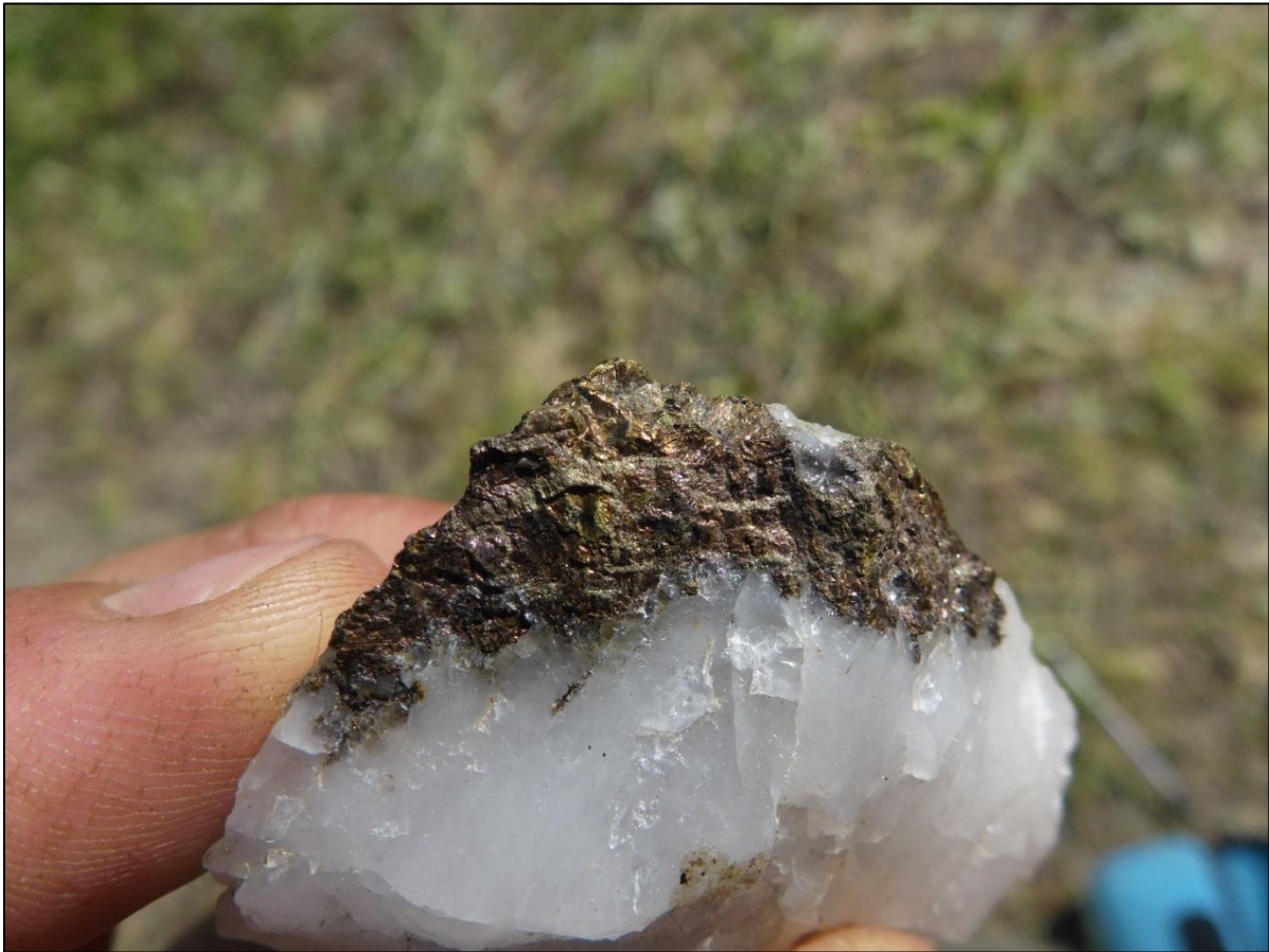
Figure 7: Representative sample collected from the Gold Standard HW 271 Showing tailings pile, displaying strong pyrite-chalcopyrite mineralization within quartz vein material.
