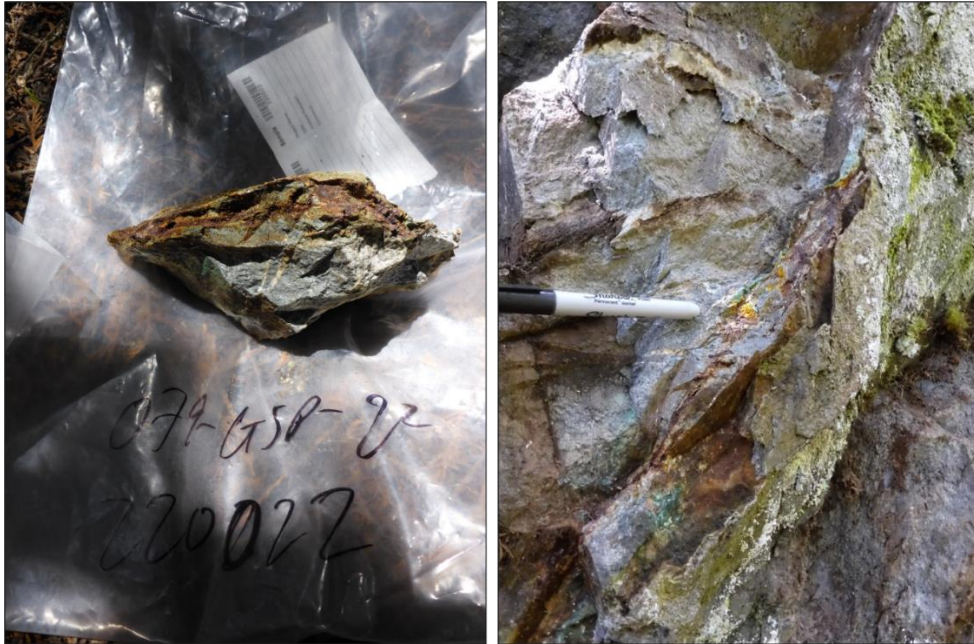
Figure 8: Sample 220022 which returned 7 ppm Au (+/- 2 ppm) within shear-related, pyrite-malachite-chalcopyrite-quartz stringers/fracturing fillings with weakly silicified intermediate volcanic wall rock.
