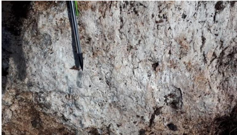
Figure 16: Saccharoidal white albitite dyke with ribbon elongate quartz, crosscut by white and purple veinlets of pollucite and lepidolite.
