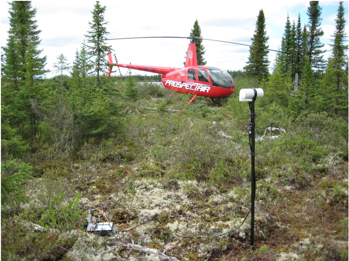
Figure 5: Example of a magnetic base station setup
