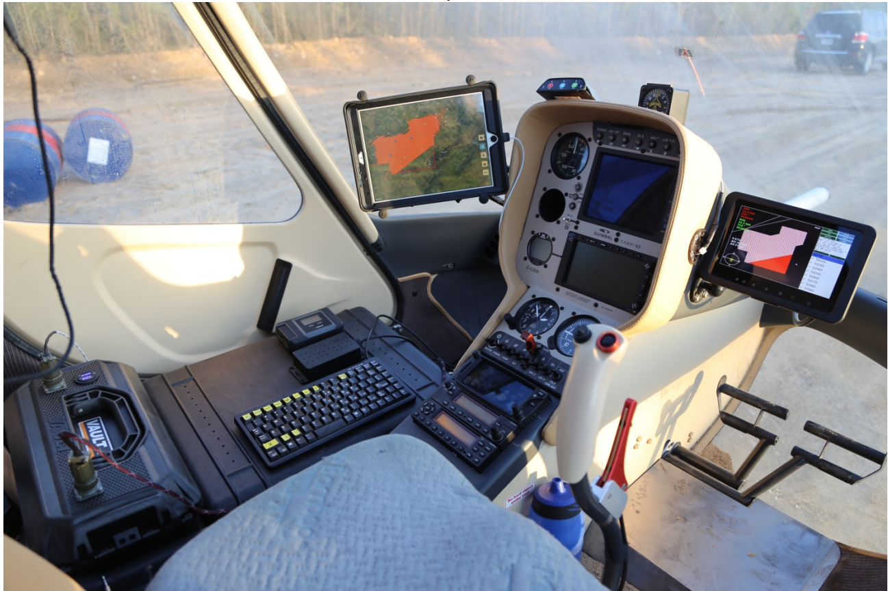
Figure 6 : Acquisition and navigation system ( SAMM ) installed in the helicopter
