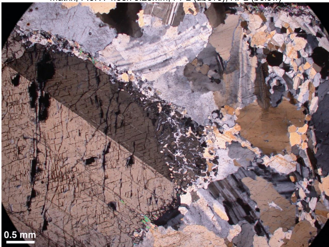
Sample 3A (2) coarse twinned spodumene and two spessartine garnet grains in qtz-albite matrix; F.o.V. 4.68x 6.25mm; PPL (above), XPL (below)
