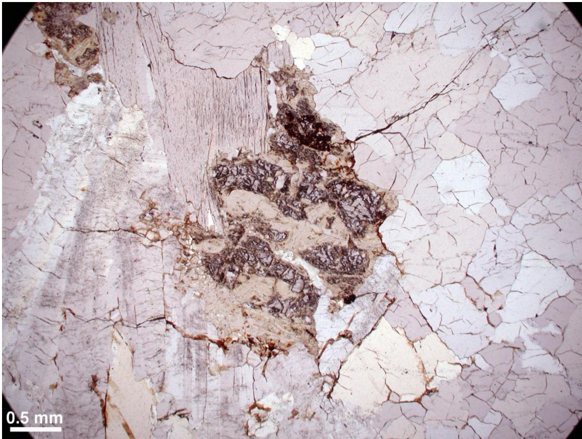
Sample 1 (1) spodumene remnants surrounded by alteration, intergrown with muscovite, plagioclase and fractured quartz; 4.50x 6.00mm; PPL (above), XPL (below)
