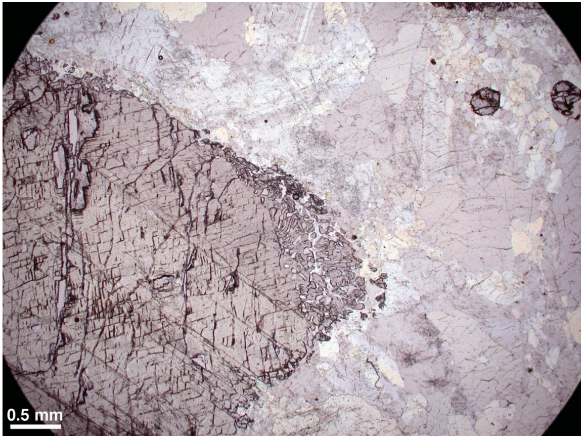
Sample 3A (2) coarse twinned spodumene and two spessartine garnet grains in qtz-albite matrix; F.o.V. 4.68x 6.25mm; PPL (above), XPL (below)
