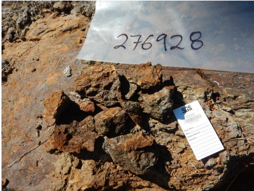
Photo 1: Sample 276928, strongly oxidized, sulphur rich, pyritic gossanous rock sample. Zone 15 498634E 5645539N (NAD83)
