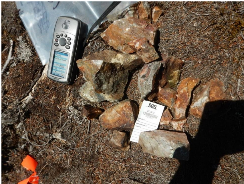
Photo 2: Sample 276931, quartz vein material from amphibolitised mafic volcanic flows believed to be within the Woman River assemblage. Zone 15 497371.2E 5645491N (NAD83)
