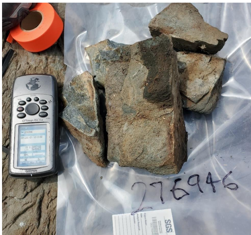
Photo 3: Sample 276946, Mafic volcanic rock, that is weakly to moderately foliated and weakly chlorite altered, light to dark green. Zone 15, 497700E 5645463N (NAD83).
