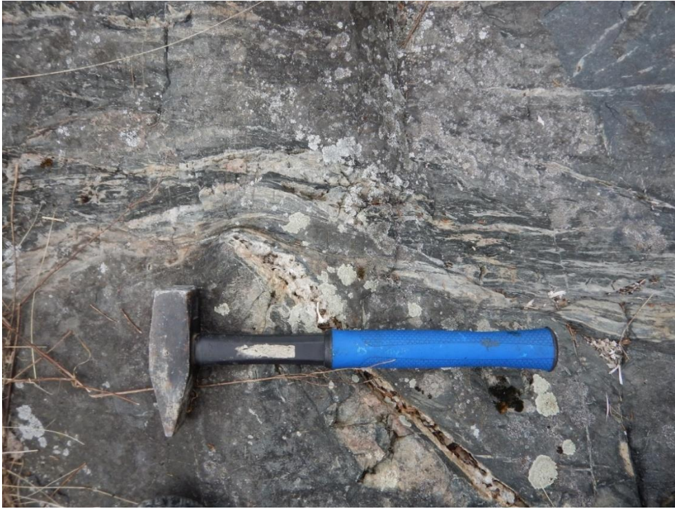
Photo 6: A strongly sheared mylonitic section trending parallel to regional foliation. Zone 15 493439E 5642832N 362Z (NAD83).
