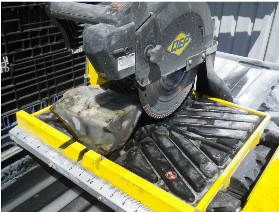
Figure 9: QEP Diamond saw and sample.
