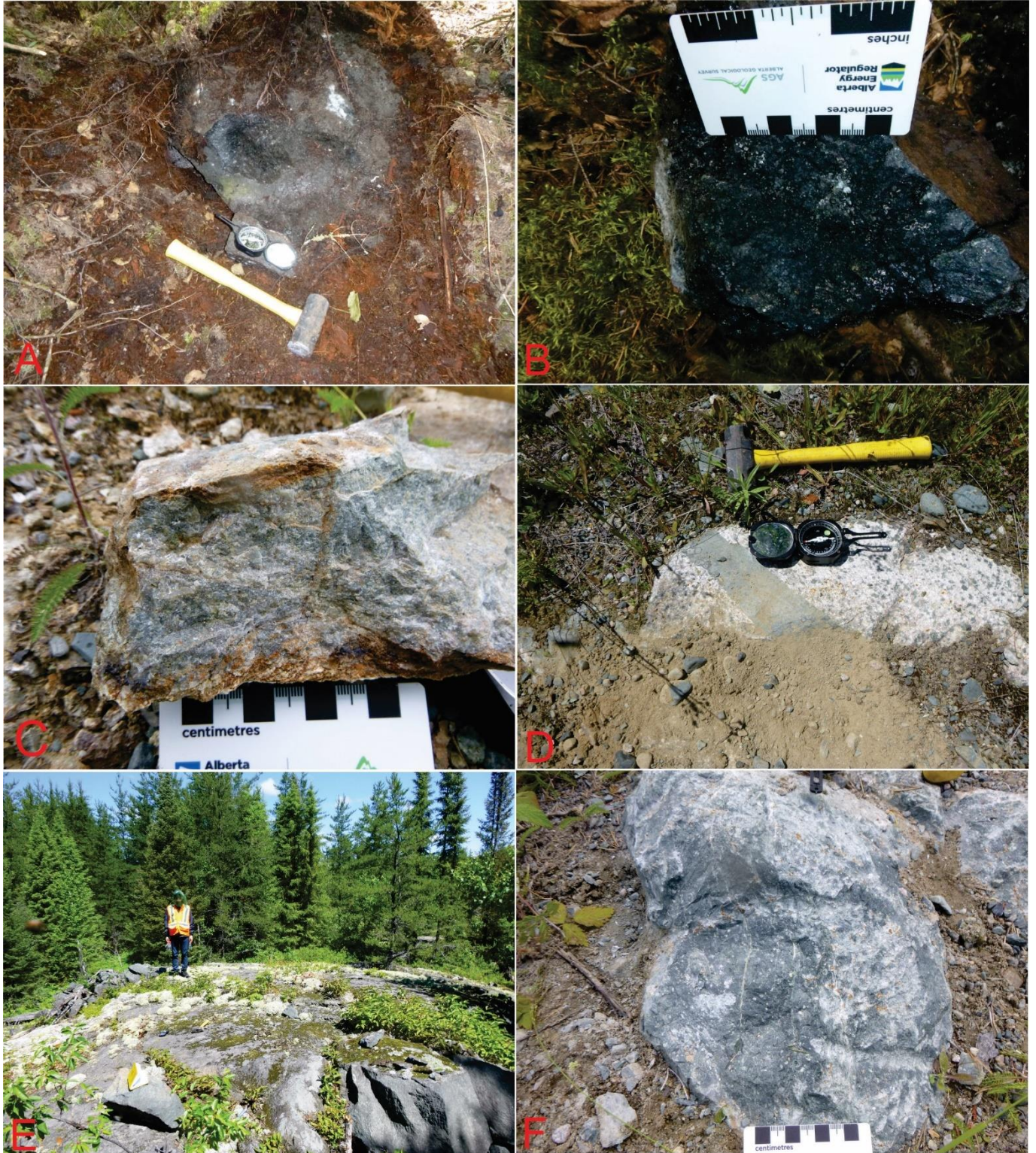
Figure 5. Photos for lithology and outcrop investigated in field. A) Outcrop of a pyroxenite intrusion. B) Sulfide minerals in pyroxenite C) Hand sample for coarse-grained anorthosite D) Outcrop for granite crosscut by a mafic dyke E) Photo of a gabbro outcrop F) Photo of a porphyritic andesite outcrop
