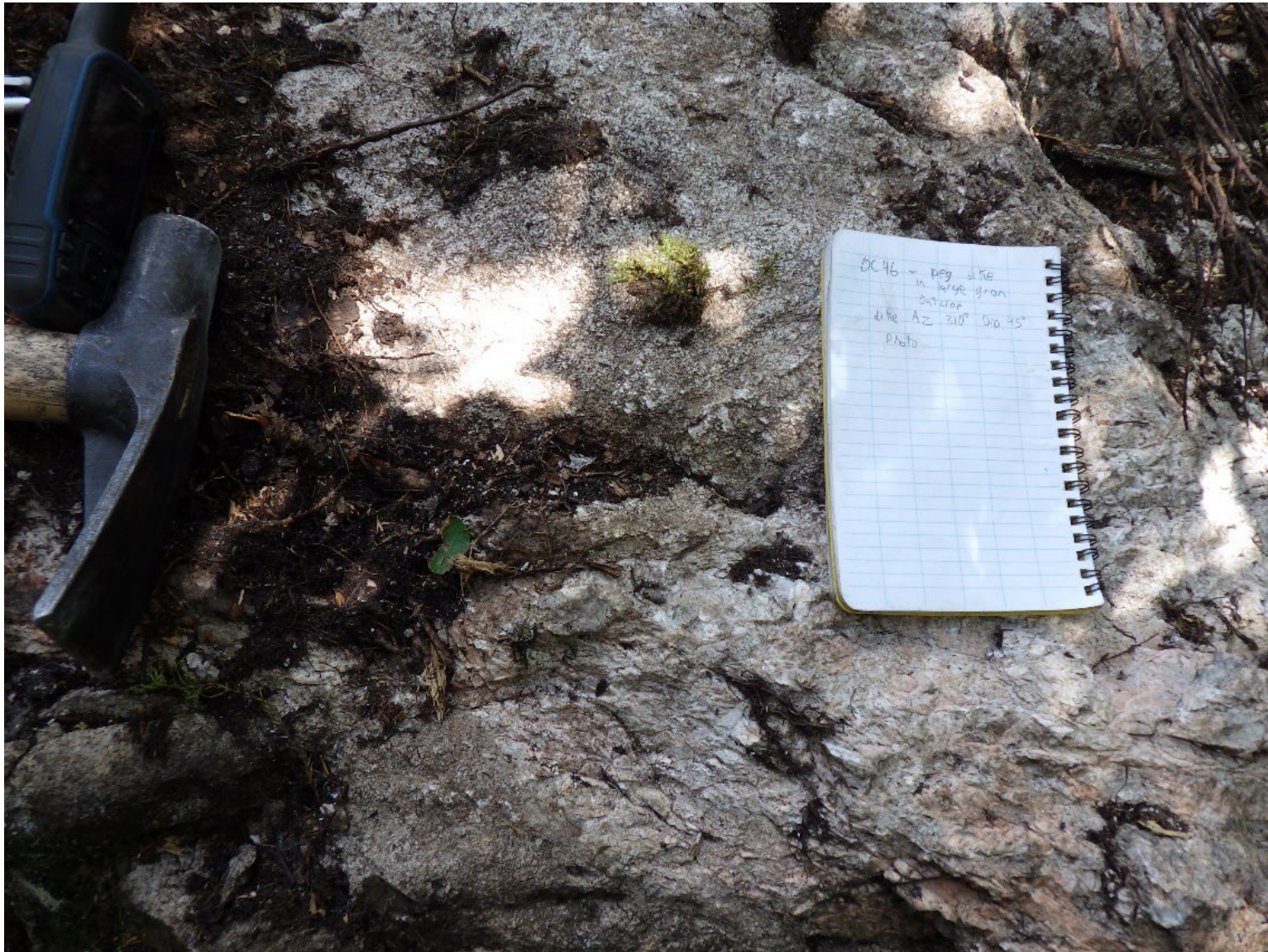
Figure 7: Outcrop 46- Contact between medium grained granite at the top of the photo, and alkaline feldspar rich pegmatite at the bottom of the photo. Contact strikes 310 degrees and dips 45 degrees to the north.
