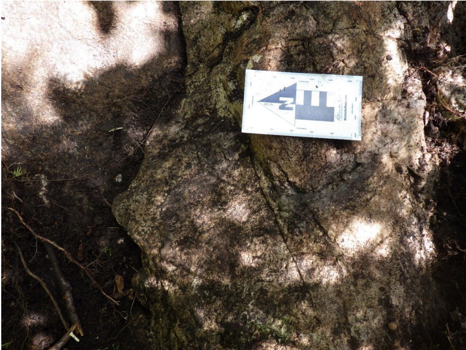
Figure 10: Outcrop 36- Contact between massive medium grained granite (right, south) and weak-moderate foliated metasediments (left, north). Contact strikes 77 degrees and has dip of 30 degrees to the south.
