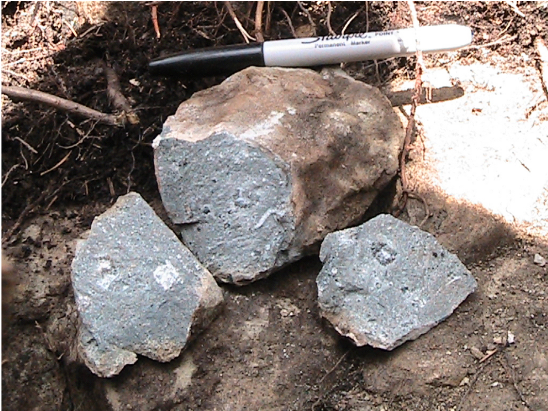
Location A - Andesitic lapilli tuff? showing chloritic and quartz shards and lapilli. Non magnetic. No reaction to 7% HCL. Located at about utm 0602682E 5363110N NAD 83. (Sharpie for scale aligned N-S, white end North)
