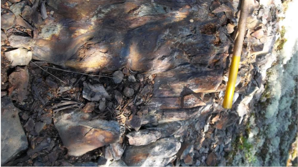
Photo 1. Strongly oxidized outcrop located west of Hamlin Lake in the northern (Hamlin grid) Sungold Property. A sample from this outcrop yielded a highly anomalous copper (up to 1.22%) and gold (up to 1570 ppb) value.
