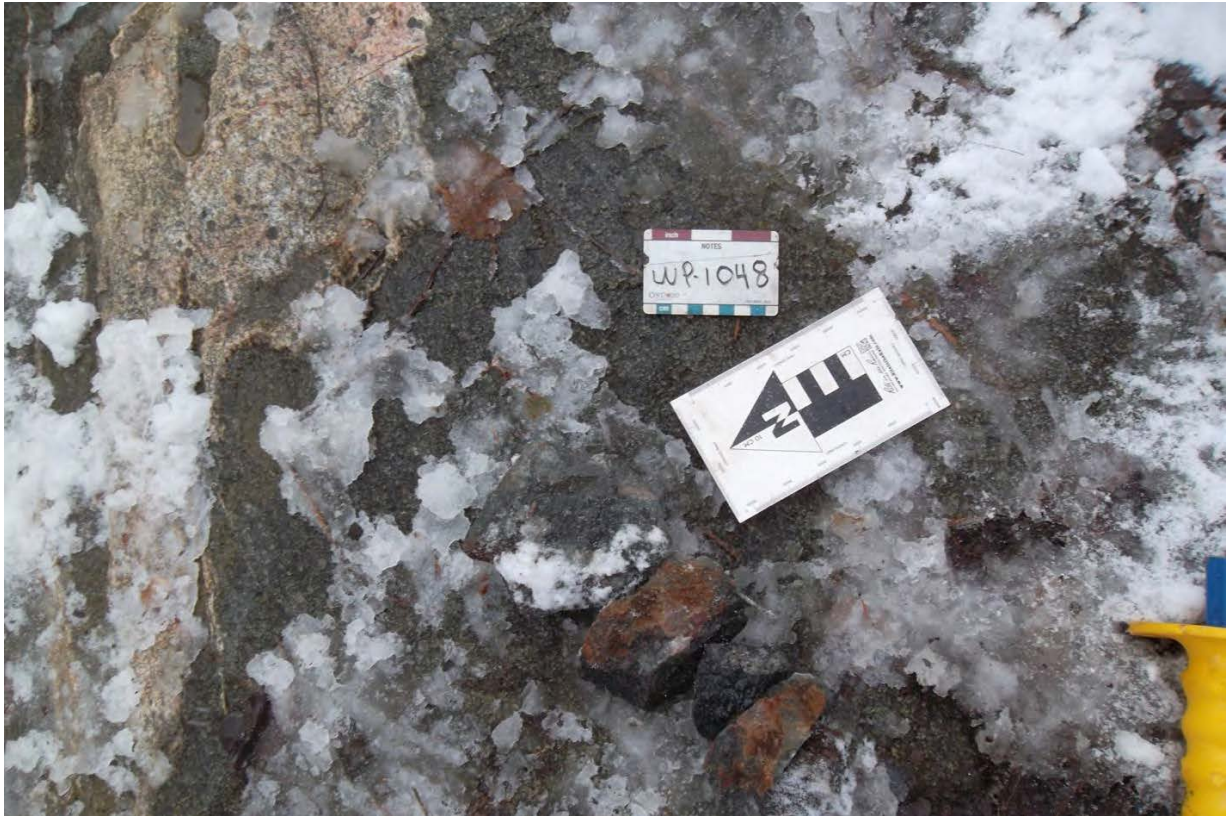
Figure 20: WP 1048: Area H - Sample E5105165 Davies Gold Occurrence closeup of biotite, quartz, pyrite alteration of mafic volcanic host rocks, found along the Ballard Lake Shear adjacent to significant quartz veining.
