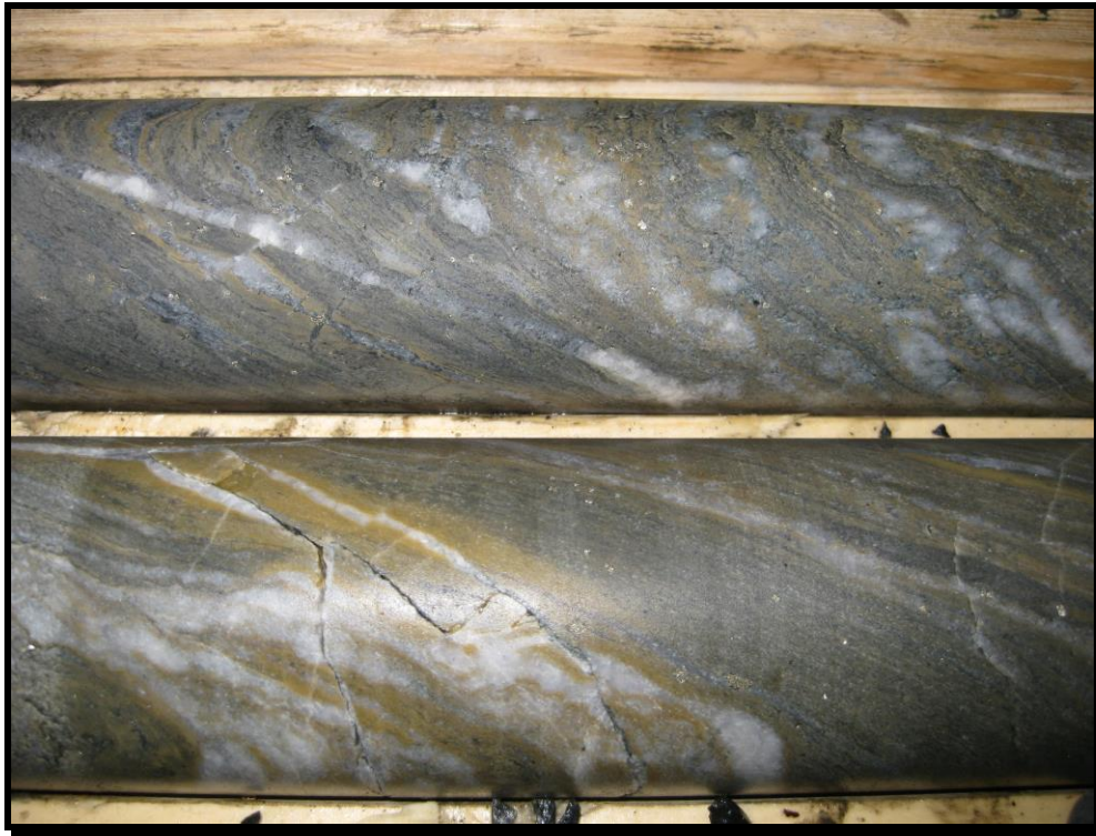
Albite-sericite-carbonate alteration typical of Thomas Ogden Zone
