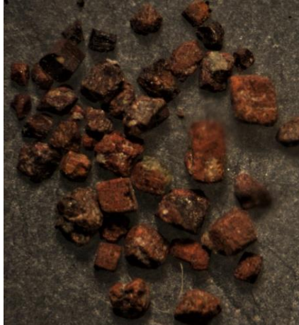
Chalcopyrite and pyrite grains
