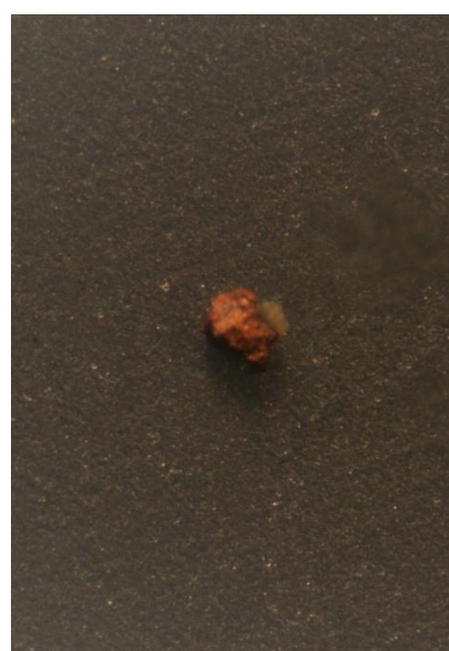
M1S Grain 6 Arsenian pyrite with quartz
