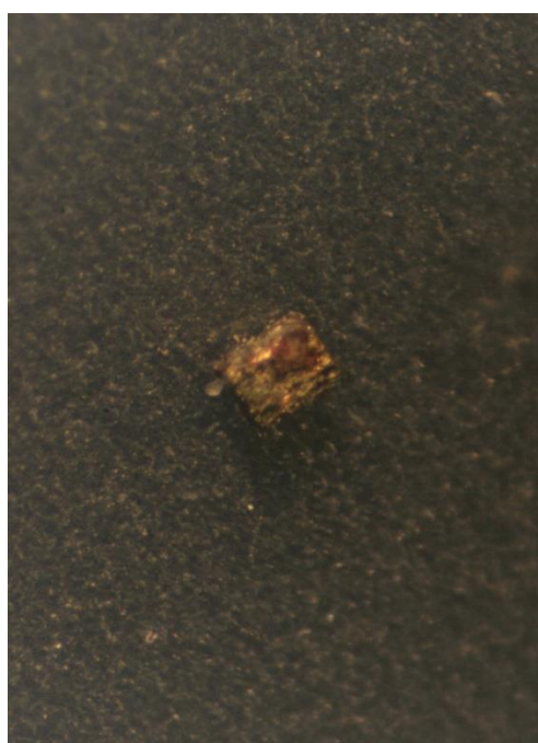
M1S Grain 8 Pyrite with chalcopyrite inclusions
