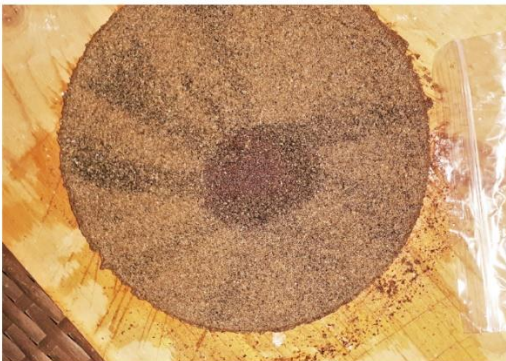
C) Heavy mineral concentrate from cable jig using a No. 80 Tyler Sieve 180 Micrometers 0.007 inches.
