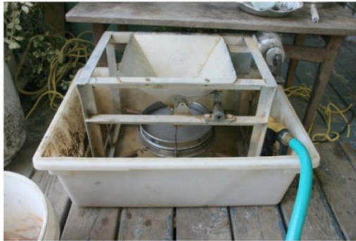
B) -1.0 mm screened fraction fed into cable jig to produce "bullseye" of heavy minerals
