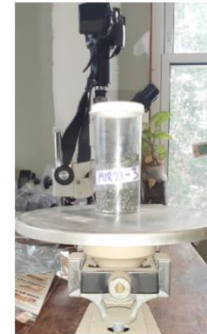
F) Concentrate is washed, dried, weighed and examined under a microscope. Minerals of interest are selected for electron microprobe analysis.
