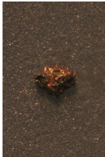
M1S Grain 3 Chalcopyrite
