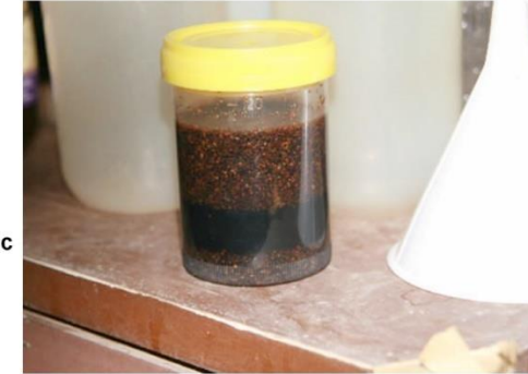
F) Concentrate is washed, dried, weighed and examined under a microscope. Minerals of interest are selected for electron microprobe analysis.
