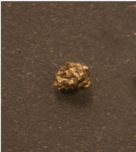
M4S Grain 7 Pyrite + chalcopyrite
