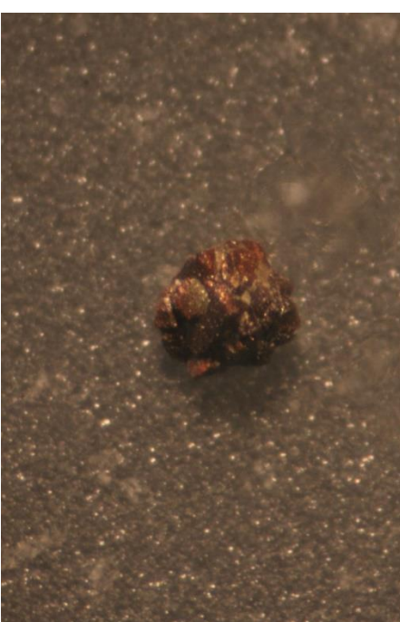
M3S Grain 8 Fe-oxide + epidote
