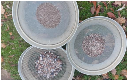
A) Samples are washed and screened
