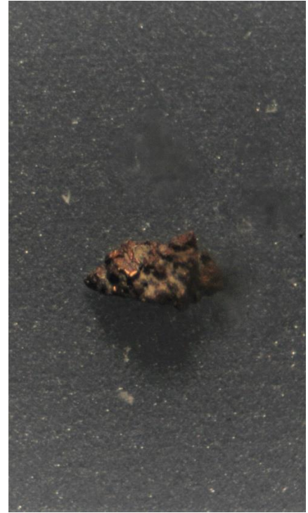
M2S Grain 3 Chalcopyrite with sphalerite
