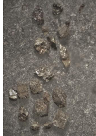
Chalcopyrite and pyrite grains
