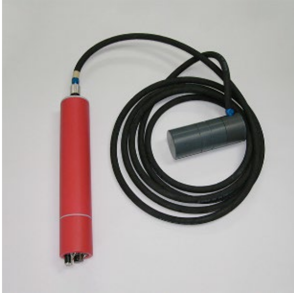
Figure 8. Scintrex CS-3 magnetometer sensor, cable, and electronics.
