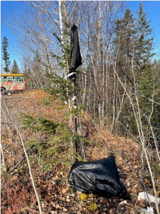
Figure 10. Base station magnetometer used for diurnal corrections.
