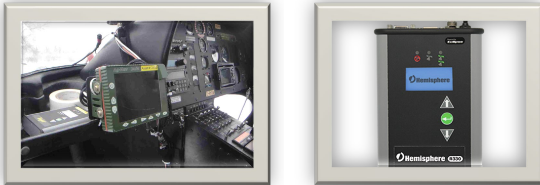
Figure 11. AgNav main console (left) and Tee-Jet GPS receiver (right).
