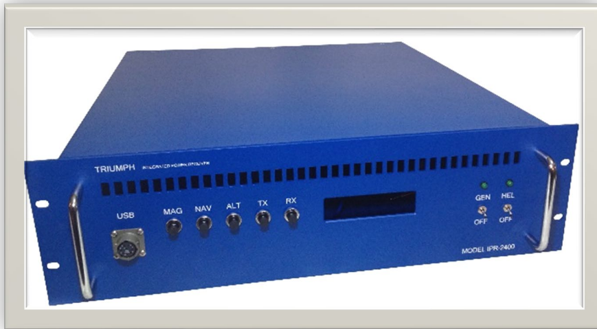
Figure 14. Triumph TDS-2400 EM console and acquisition system.
