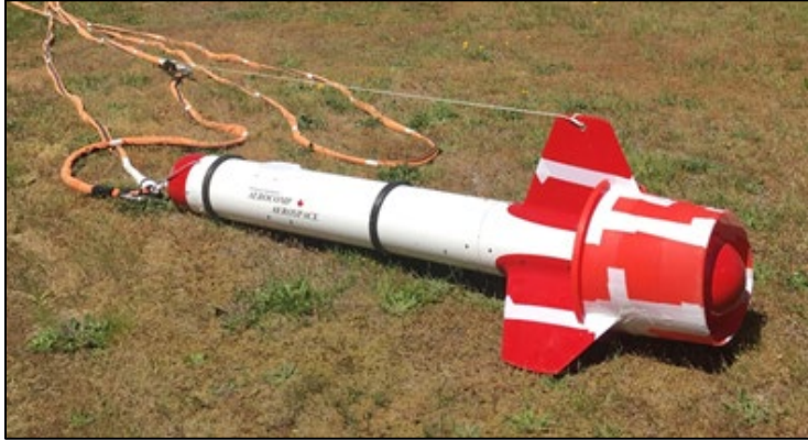
Figure 9. Airborne magnetometer housing with tow cable.
