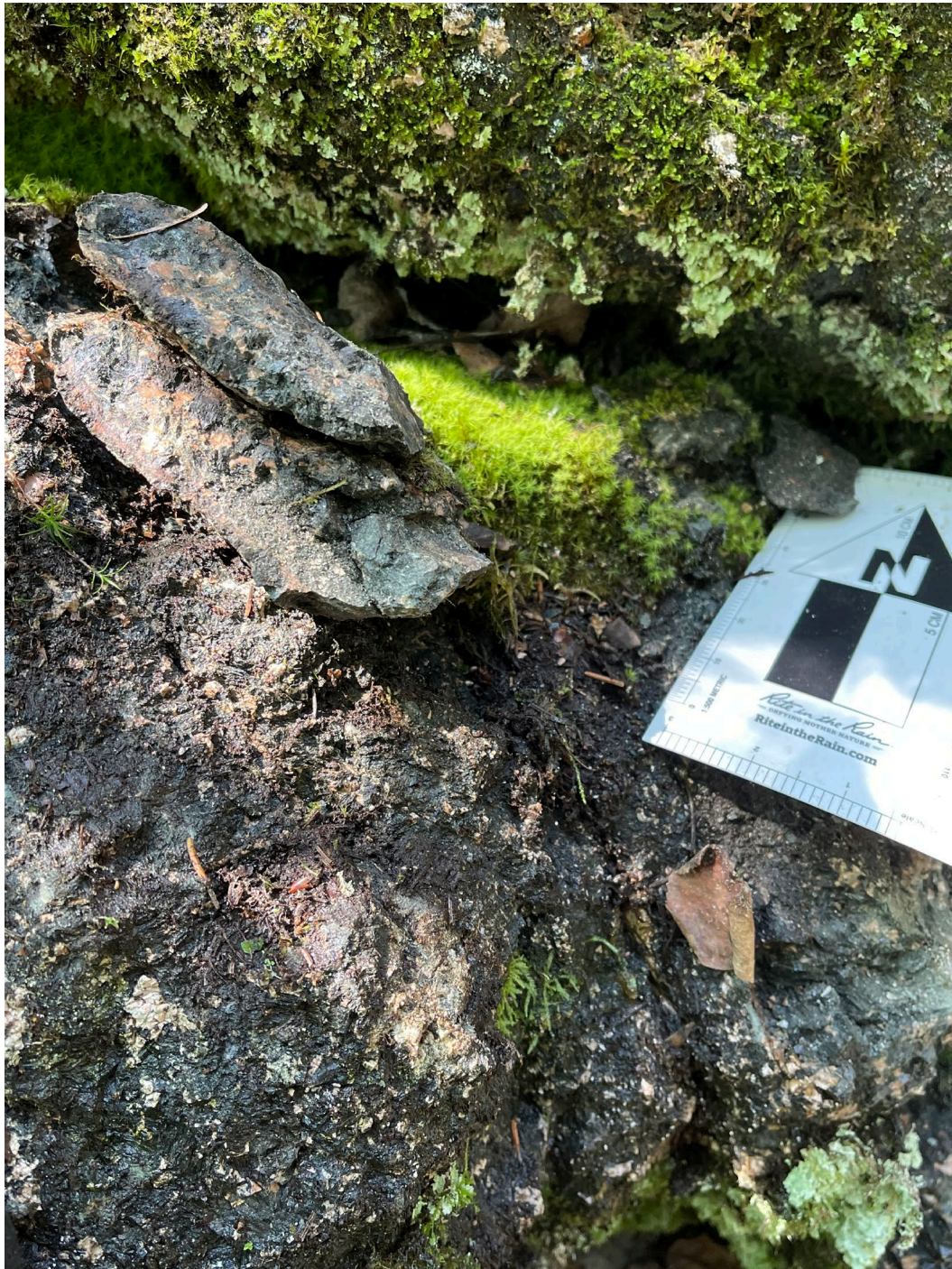
PhotoPlate 1: POI-JC-027_NW (NAD83 Zn16 532,514E 5,415,644N) outcropping of tourmaline-amphibole and K-feldspar pods within syenite outcrops along the Little Pic River. Pods were found to have sporadic weak to moderate magnetism, with magnetite occurring as an accessory mineral. No sulphides were observed within the pods.
