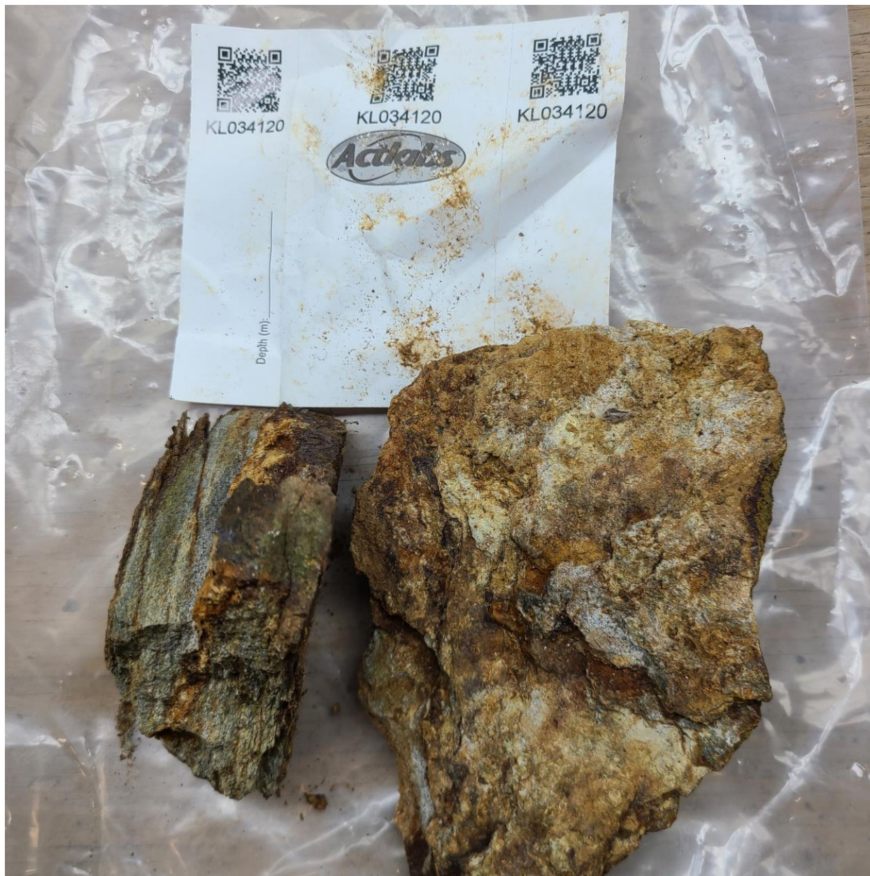
Figure 7: Sample KL034120 of Chlorite Schist with 0.587 g/t Au and 1.63% As.
