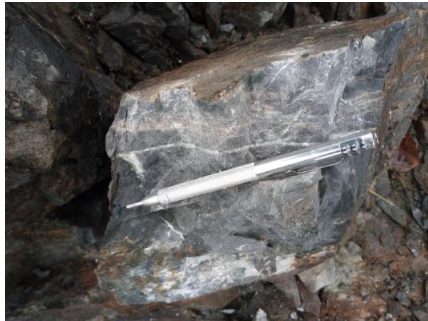
Trench A: Quartz stringers in basalt, northeast section. 594778mE, 5367268mN
