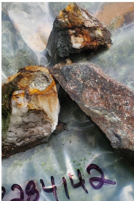
Figure 2: Red alteration and heavy mineralisation in sample B284142
