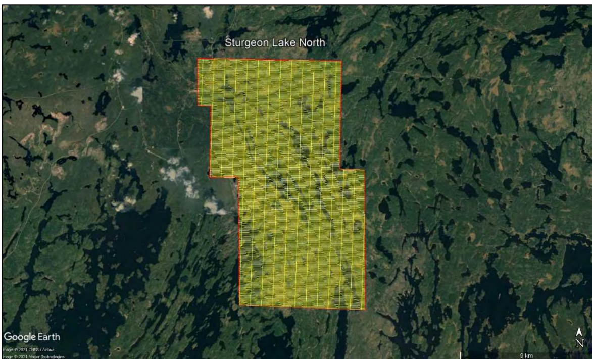
Figure 3: Plan View – Sturgeon Lake North block with actual flight lines in yellow and survey block boundary in red.
