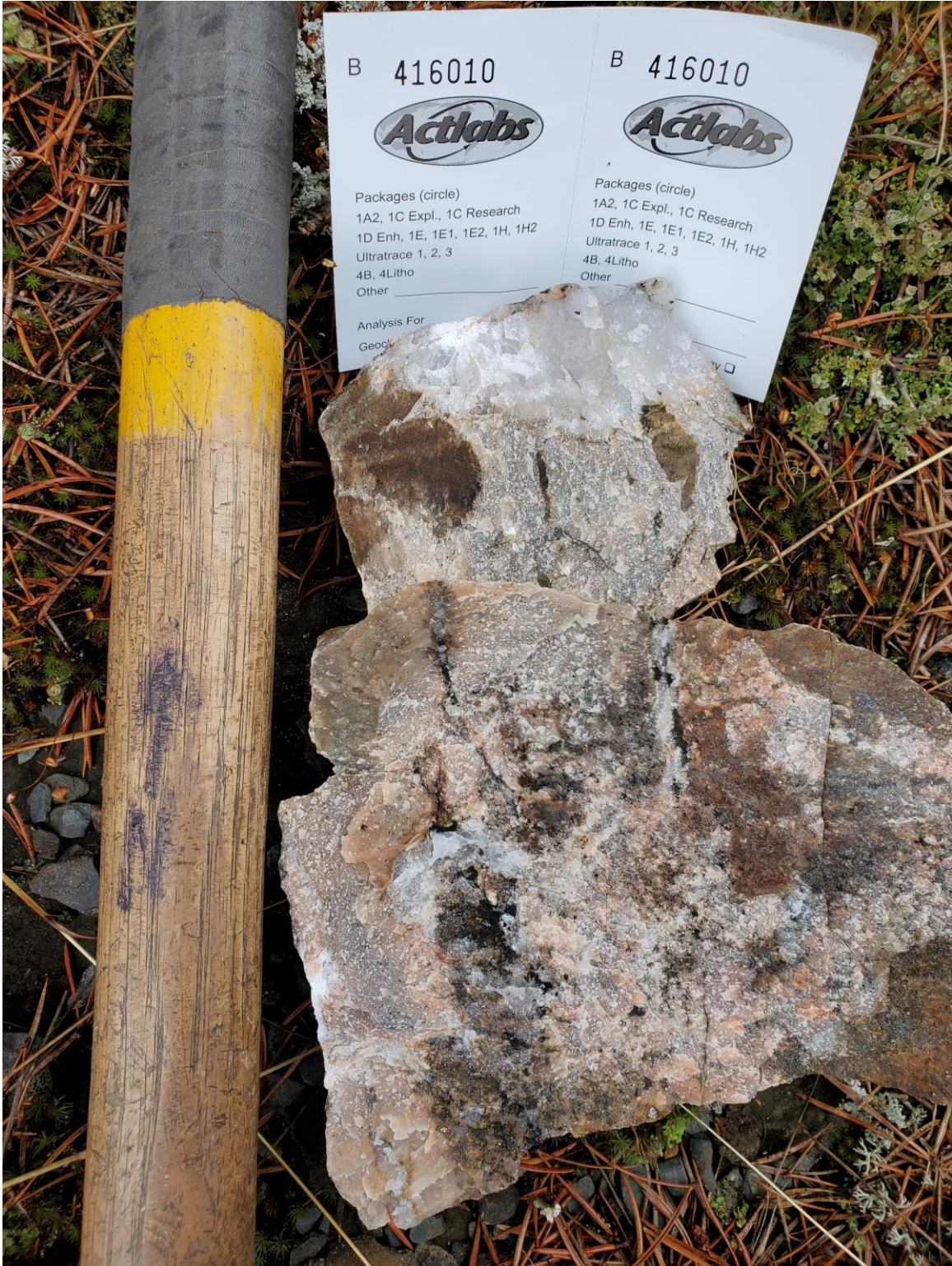
Sample B416010: Angular float of brecciated felsic-cherty rock with quartz veining, pyrite, goethite. Burchell property, hand sample, view to N.
