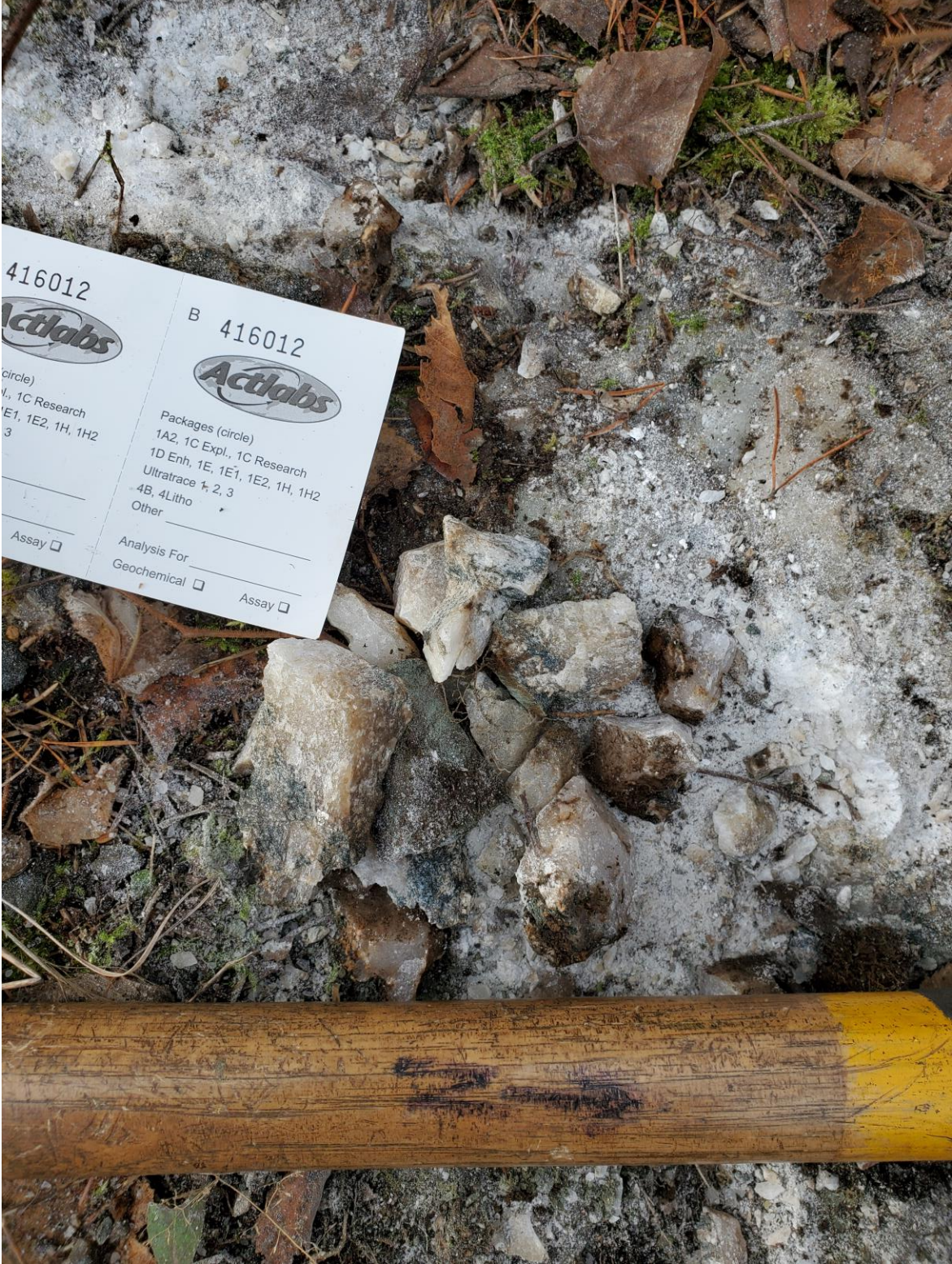
Sample B416012: Qtz in brecciated mafic-felsic contact, py-cubes, actinolite, qzt-sugary texture (near POI_DR_471 on road).
