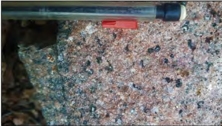
Figure 11: Vuggy, carbonate altered granite with biotite/calcite/pyrite/chalcopyrite in void spaces (JK-SF-016)
