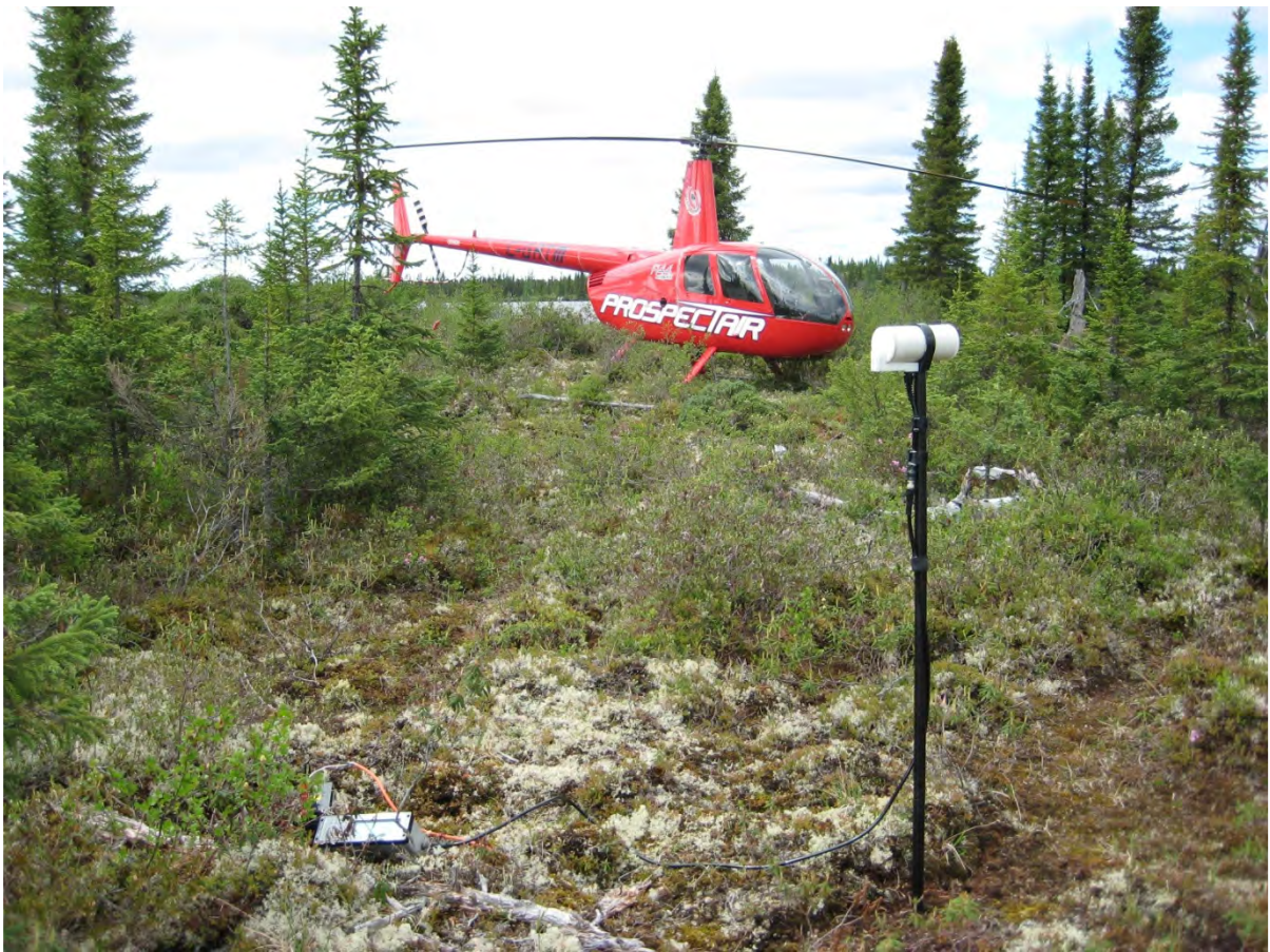
Figure 5: Example of a magnetic base station setup
