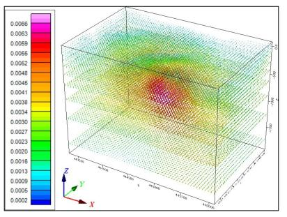
Figure 25: VOXI Fine MVI vector voxel magnetization model.
