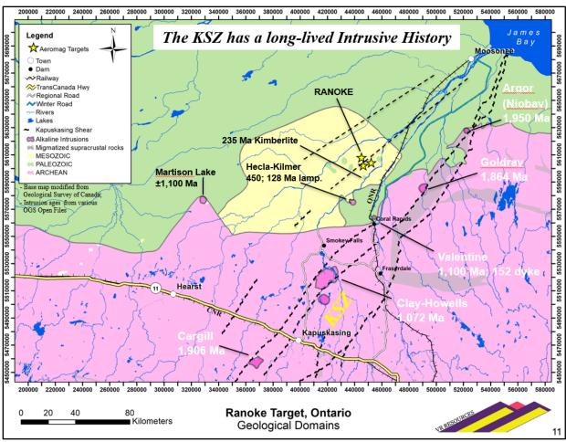
Figure 2: Regional geology map of Kapuskasing structural zone (KSZ) and James Bay Lowlands with alkaline and ultrabasic intrusions and their ages highlighted. The Northway target is noted by 3 gold stars indicating magnetic targets.
