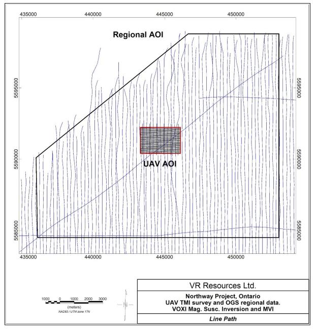
Figure 1: The linepath for the surveys (blue is regional and black is UAV) and the AOIs (black is regional and red is detailed UAV) .
