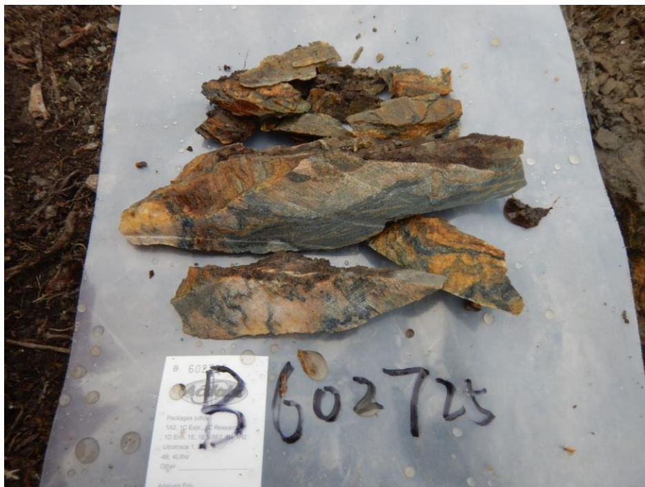
Photo 2: Sample B602725 collected within the <30 cm shear zone from outcrop 2. Assay value 0.513 g/t Au.
