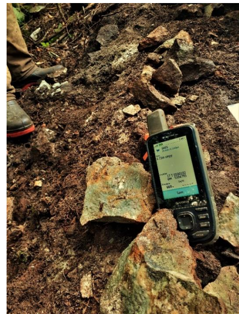
Waypoint 405, ML22-97 0.131 ppm Au, 2,270 ppm Ni, 374 ppm Co, 48 ppm Sb 500102mE, 5304795mN
