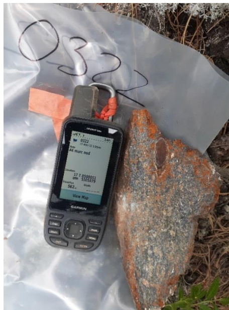
Waypoint 322, ML22-80 0.034 ppm Au, 643 ppm Ni, 66.8 ppm Co, 34 ppm Sb 500051mE, 5305079mN
