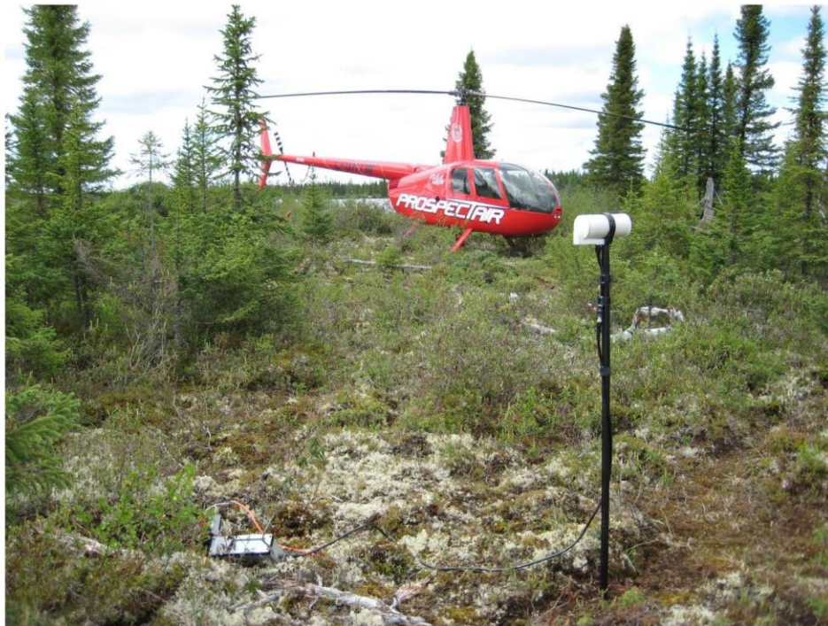
Figure 5: Example of a magnetic base station setup
