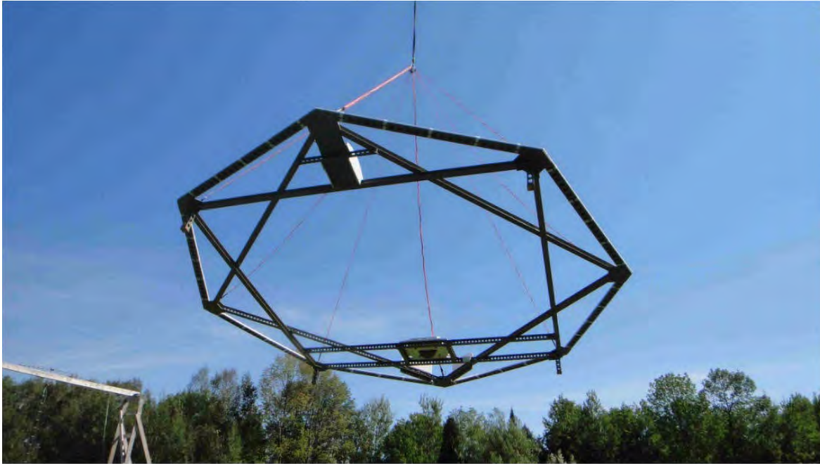
Figure 6. The Triumph AirTEM™ TS-150 HTEM System.
