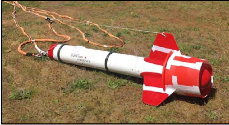
Figure 9. Airborne magnetometer housing with tow cable.
