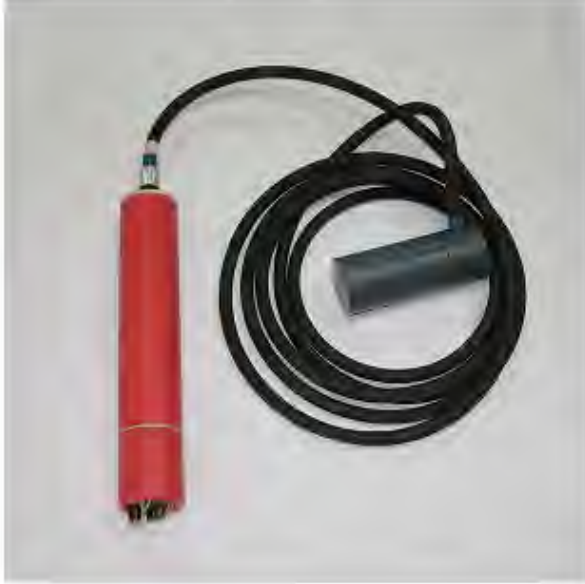
Figure 8. Scintrex CS-3 magnetometer sensor, cable, and electronics.
