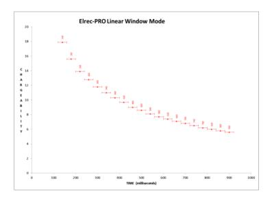
Figure 16. Linear windows (1 s pulse) after windowing of the fullwaveform recorded signal.
