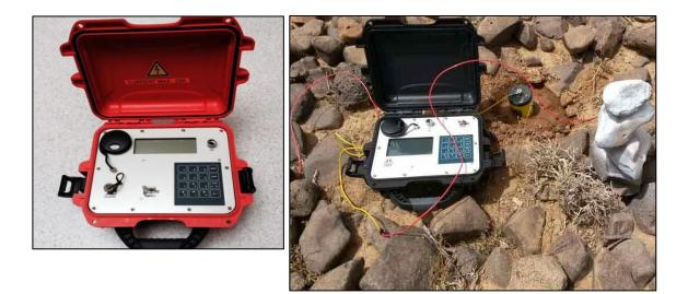
Figure 4. I-Fullwaver (left) and V-Fullwaver (right) from IRIS Instruments.
