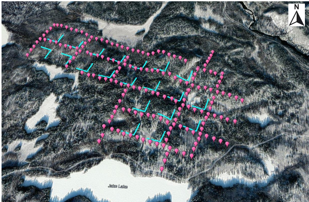
Figure 19: Topographical Relief with the Survey Deployment for West Setup Looking Northwest (©2022 Google, Image ©2022 CNES/Airbus)
