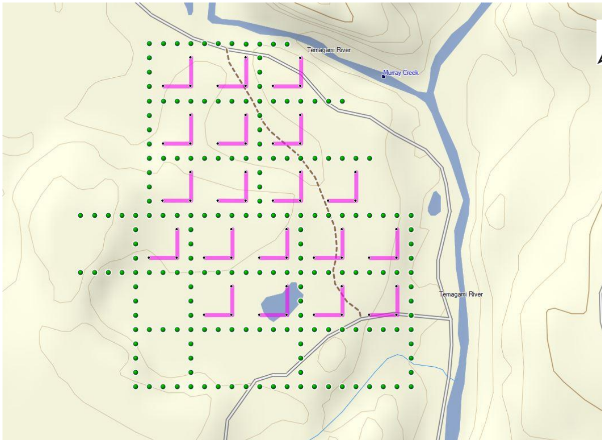
Figure 8: Planned Survey Layout for North Setup – Green Circles =Current Injections, Pink Lines=Dipoles, Black Dots=Read Electrodes
