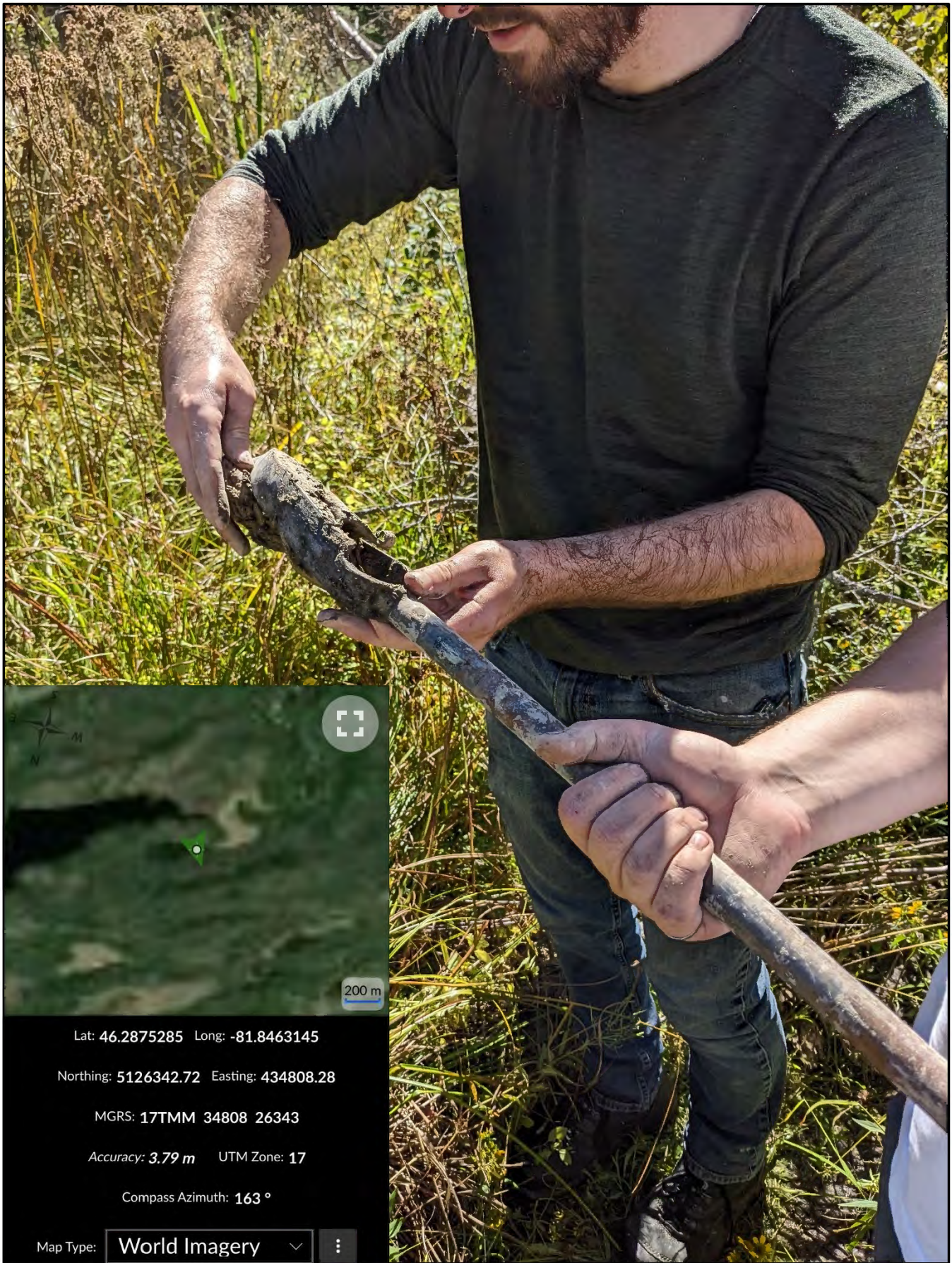
Figure 6 STATION 4. RETRIEVING CLAY FROM SOIL AUGER IN SWAMP-GRASSLAND AREA IMMEDIATELY EAST OF BEAVER DAM.
