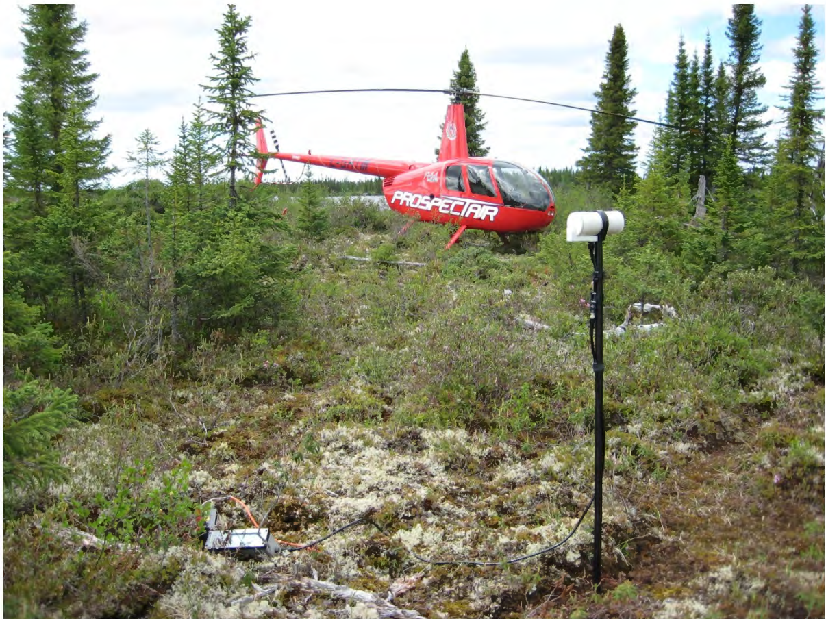
Figure 6: Example of a magnetic base station setup
