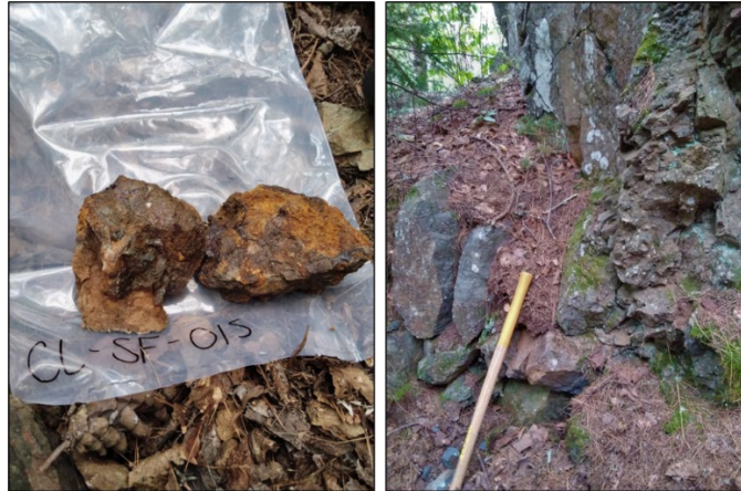
Figure 8: Grab sample D579664 returned values of 0.26% Cu, 0.12% Ni, with negligible Pt and Pd concentrations from a strongly oxidized piece of gabbro float with 20-25% disseminated pyrrhotite-lesser chalcopyrite located in the southwest portion of the property near the Arrow River target area.
