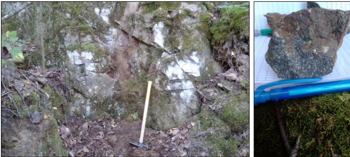
Figure 9: Sample D579694 which returned values of 0.21% Cu, 0.17% Ni, and low Pt and Pd concentrations from gossanous gabbro containing up to 2% disseminated pyrite-lesser-pyrrhotite-chalcopyrite collected from the Central Bearpad Lake target area, near the Crystal Lake Gabbro junction.
