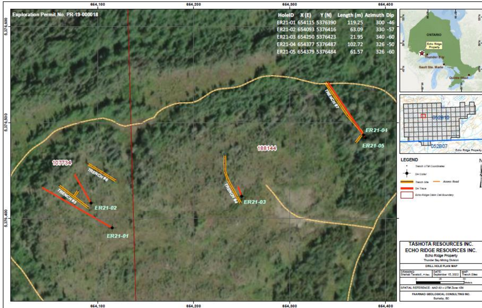
Figure 12. Enlarged map area showing the five 2021 drill holes (ER21-01 to ET2105) targeting observed mineralization at depth in the trenches ET-4, ET-5, and ET-7.
