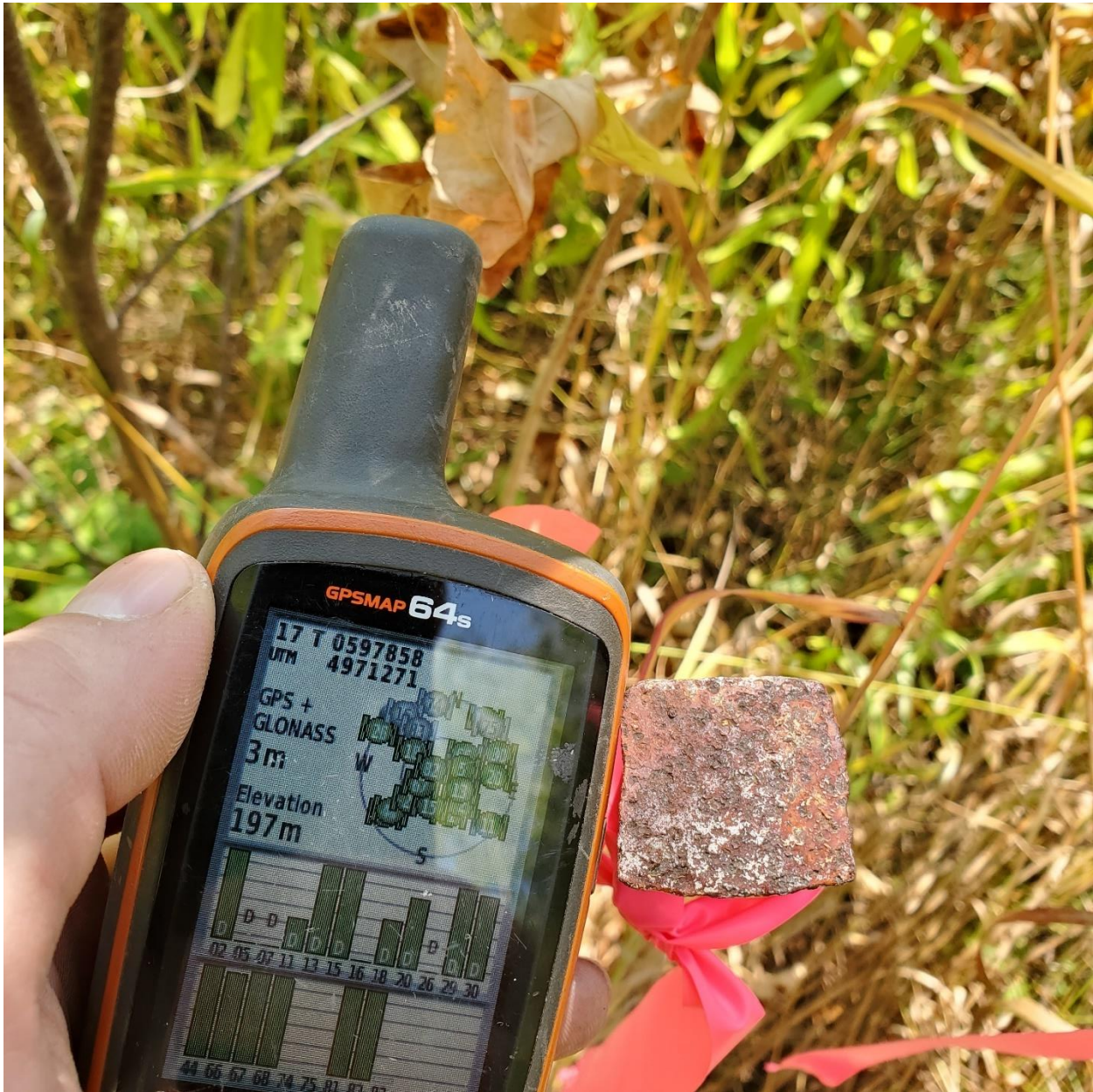
Figure 5: Survey Bar Located
