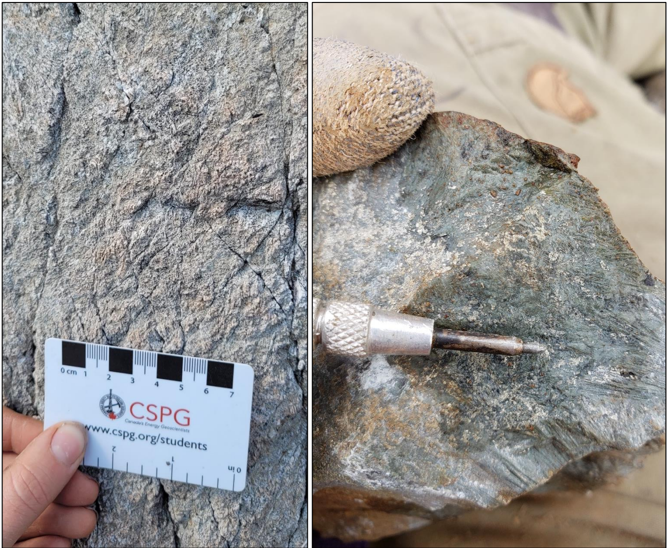
Figure 27. Spinifex texture seen on outcrop and hand sample.
