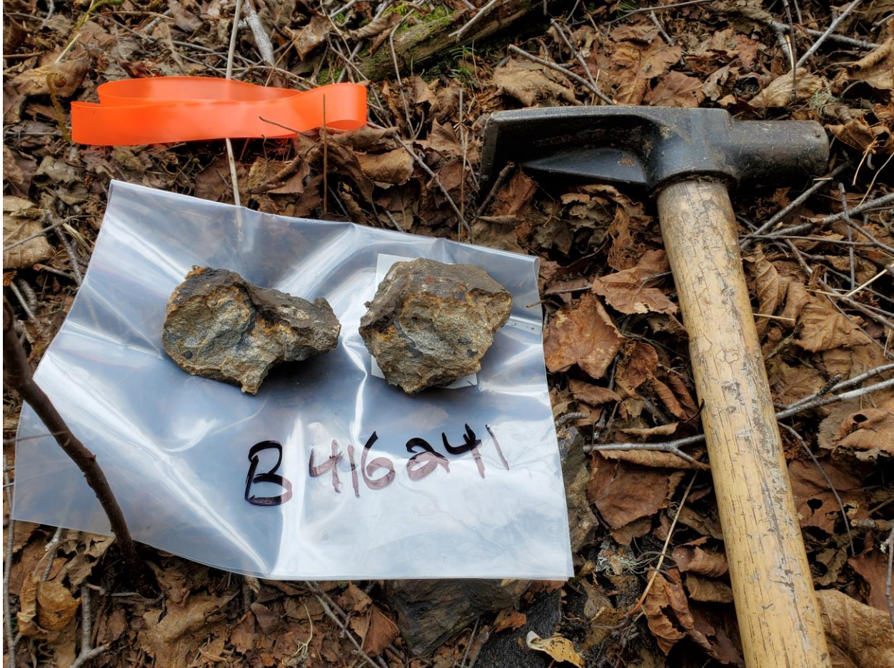
Sample B416241 – 1.36% Zn, 635 ppm Pb, 11.6 ppm Ag
